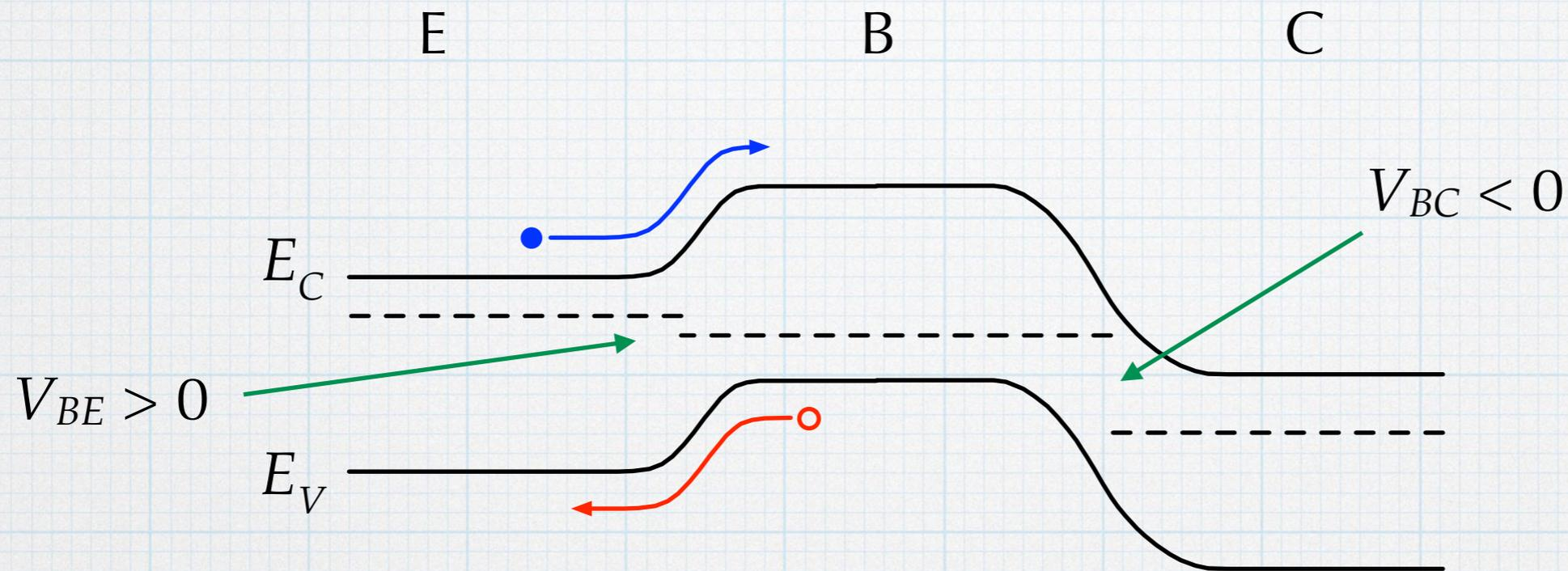
Electrons and holes will be injected across the base-emitter junction.
