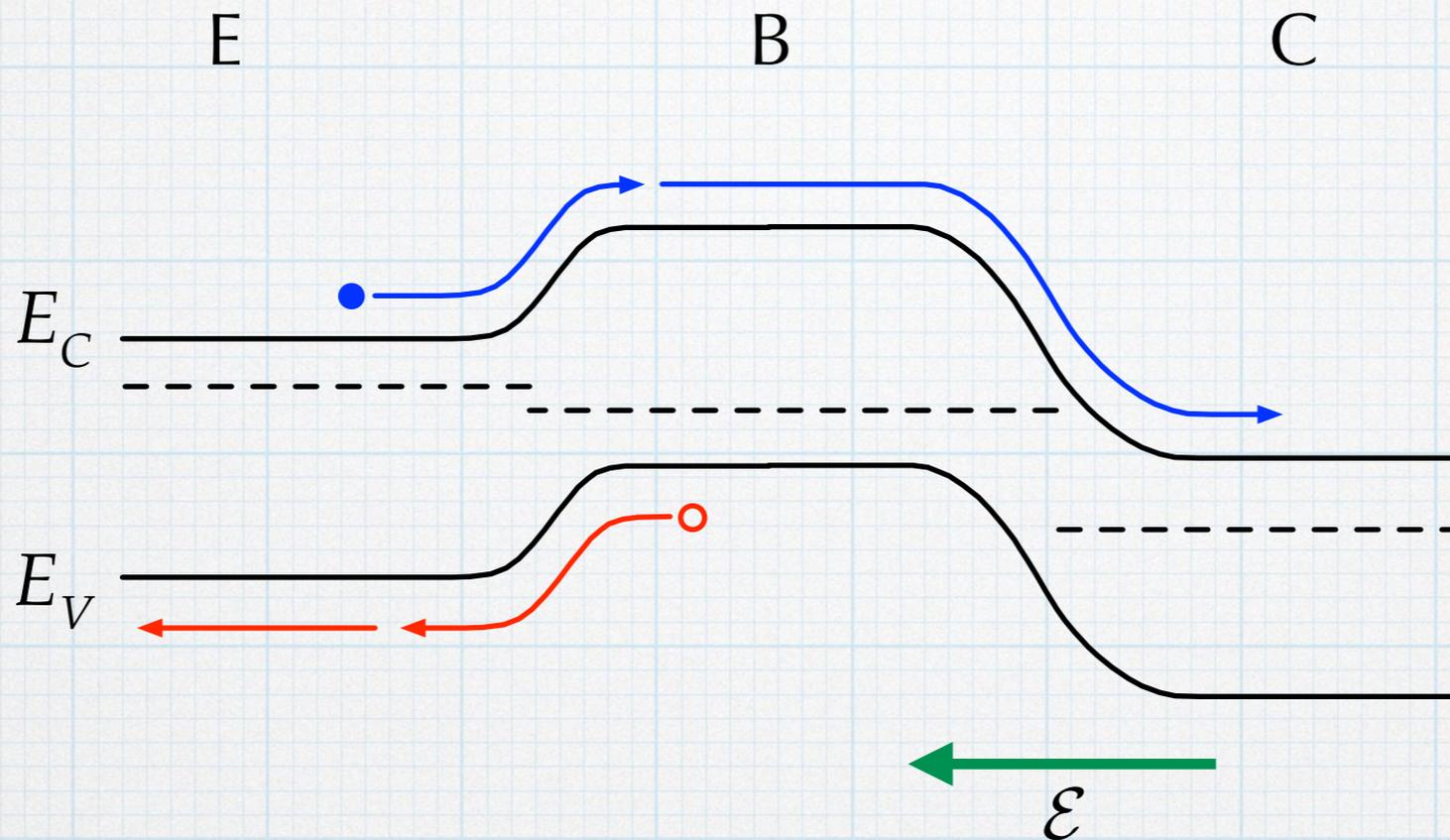
The electrons will diffuse across the base region. When they get to the high electric field at the B-C, they will be swept across and into the collector. They end up as collector current!
