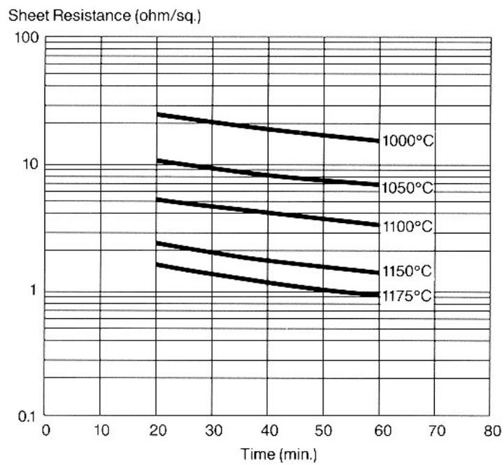
**Figure 3C. Sheet Resistance vs. Deposition Time and Temperature for BN-1100 and BN-1250**
