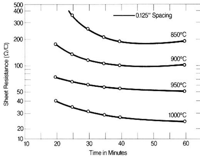
**Figure 3B. Sheet Resistance vs. Deposition Time and Temperature for BN-HT**
