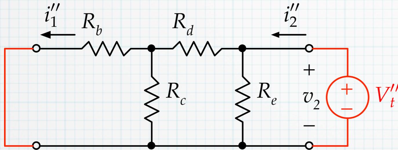
$$i''_2 = \frac{V'_t}{R_{eq}} = \frac{V'_t}{R_e \parallel [R_d + R_c \parallel R_b]}$$
