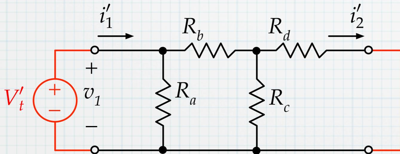
$$i'_1 = \frac{V'_t}{R_{eq}} = \frac{V'_t}{R_a \parallel [R_b + R_c \parallel R_d]}$$
