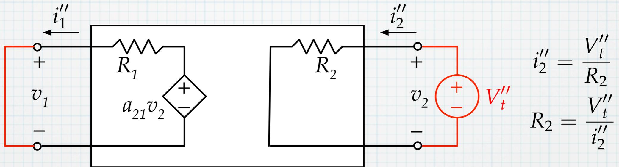
$$i_1'' = \frac{a_{21} V_t''}{R_1} \quad \frac{R_1}{a_{21}} = \frac{V_t''}{i_1''}$$
