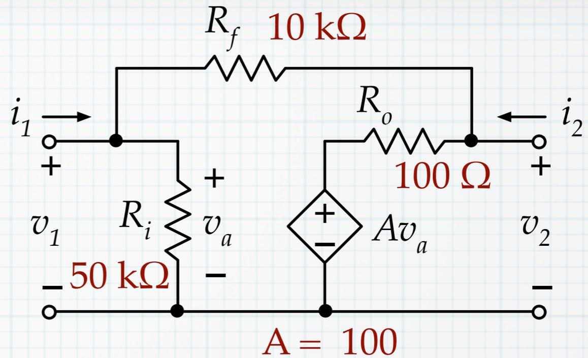
1. Apply a test voltage at  $v_1$ . Short circuit  $v_2$ . Calculate the terminal currents.
