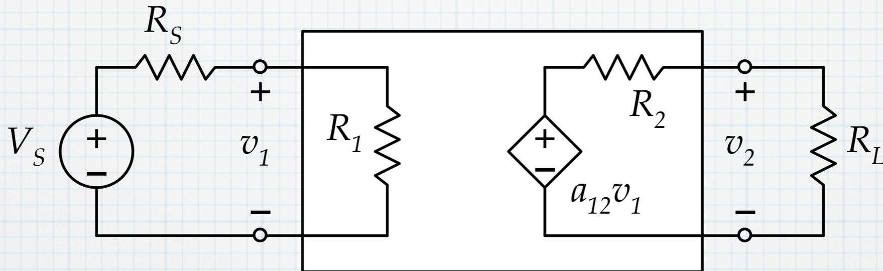
$$v_1 = \frac{R_1}{R_1 + R_S} V_S$$
