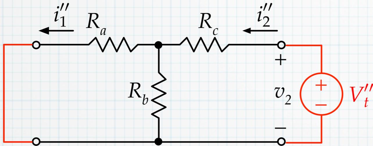
$$i''_2 = \frac{V''_t}{R_{eq}} = \frac{V''_t}{R_c + R_a \parallel R_b}$$
