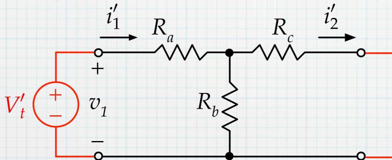
$$i'_1 = \frac{V'_t}{R_{eq}} = \frac{V'_t}{R_a + R_b \parallel R_c}$$
