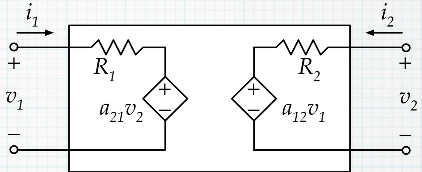
1. Apply a test voltage,  $V_t'$  at port 1.  $v_1 = V_t'$ .
