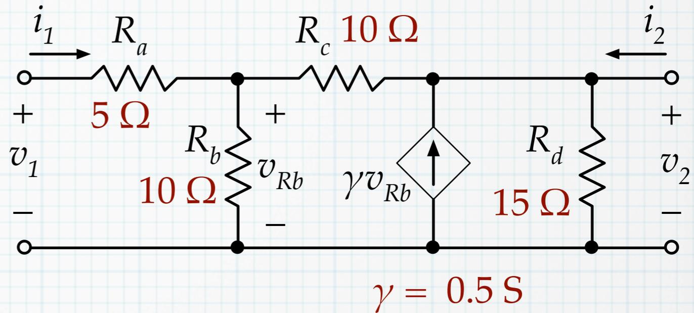
1. Short circuit  $v_2$ . ( $R_d$  is shorted out.) Apply a test voltage at  $v_1$ . Calculate the terminal currents.
