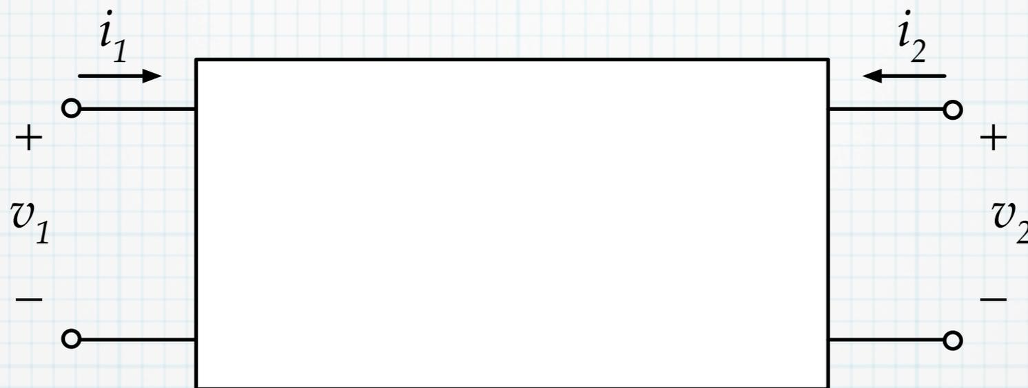
The form of two-port equivalent that we have used to this point is just one of several different forms. There are other ways to view the relationship between the terminal currents and voltages. What we have done is to write the currents in terms of the voltages.
