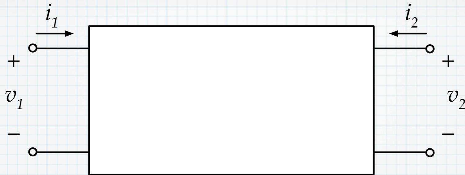
Express  $v_1$  and  $i_2$  terms of  $v_2$  and  $i_1$  (hybrid parameters)
