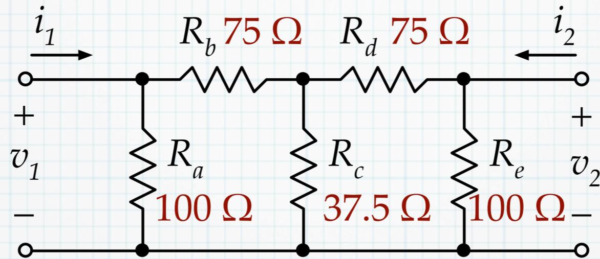
1. Apply a test voltage at  $v_1$ . Short circuit  $v_2$ . ( $R_e$  is shorted out.) Calculate the terminal currents.
