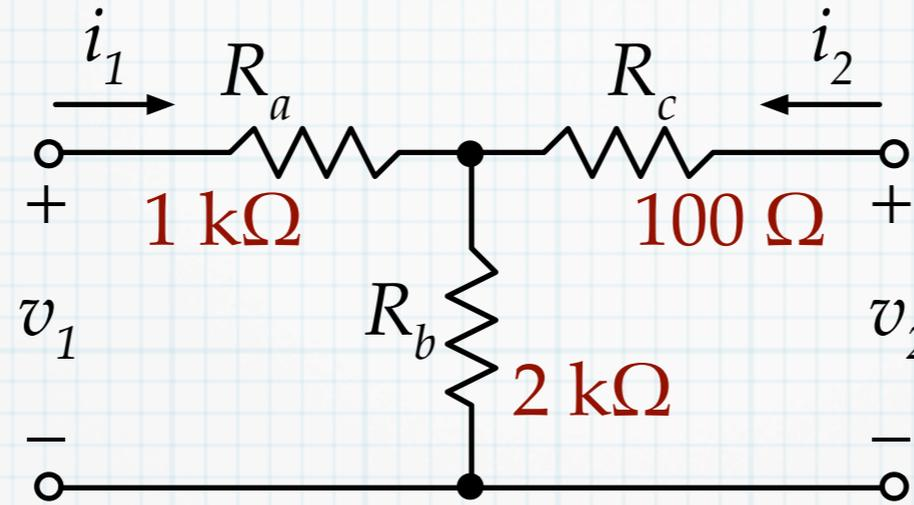
1. Apply a test voltage at  $v_1$ . Short circuit  $v_2$ . Calculate the terminal currents.
