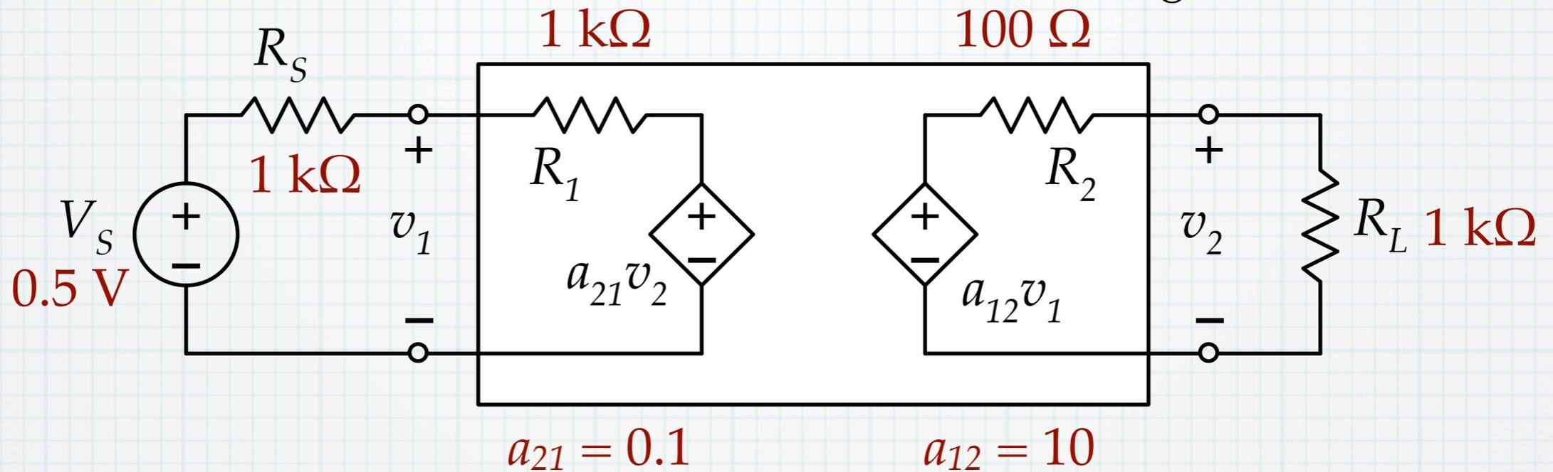
$$v_2 = \frac{R_L}{R_L + R_2} a_{12} v_1 \quad \longrightarrow \quad v_1 = \frac{R_L + R_2}{R_L} \frac{v_2}{a_{12}}$$
