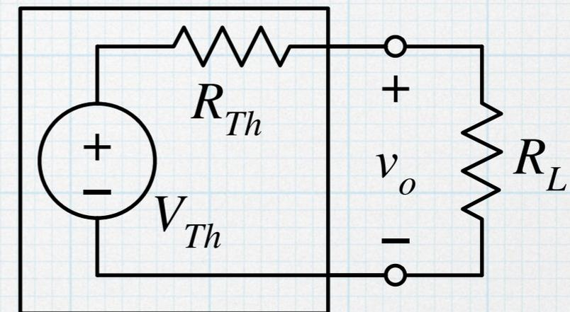
If we view the power as a function of  $R_L$ , we can find the maximum by using the usual calculus trick of taking the derivative and setting it equal to zero.
