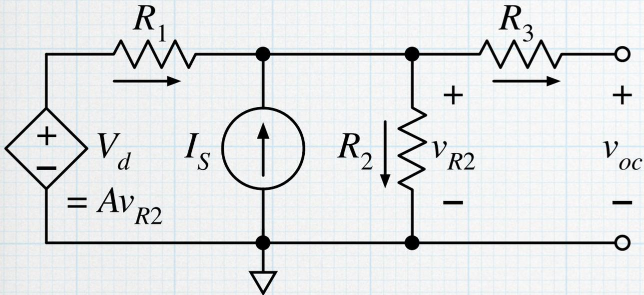
Find  $v_{oc}$ , which is equal to  $v_{R2}$ .
