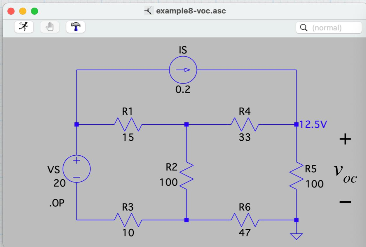
$$V_{Th} = v_{oc} = 12.5 \text{ V.}$$
