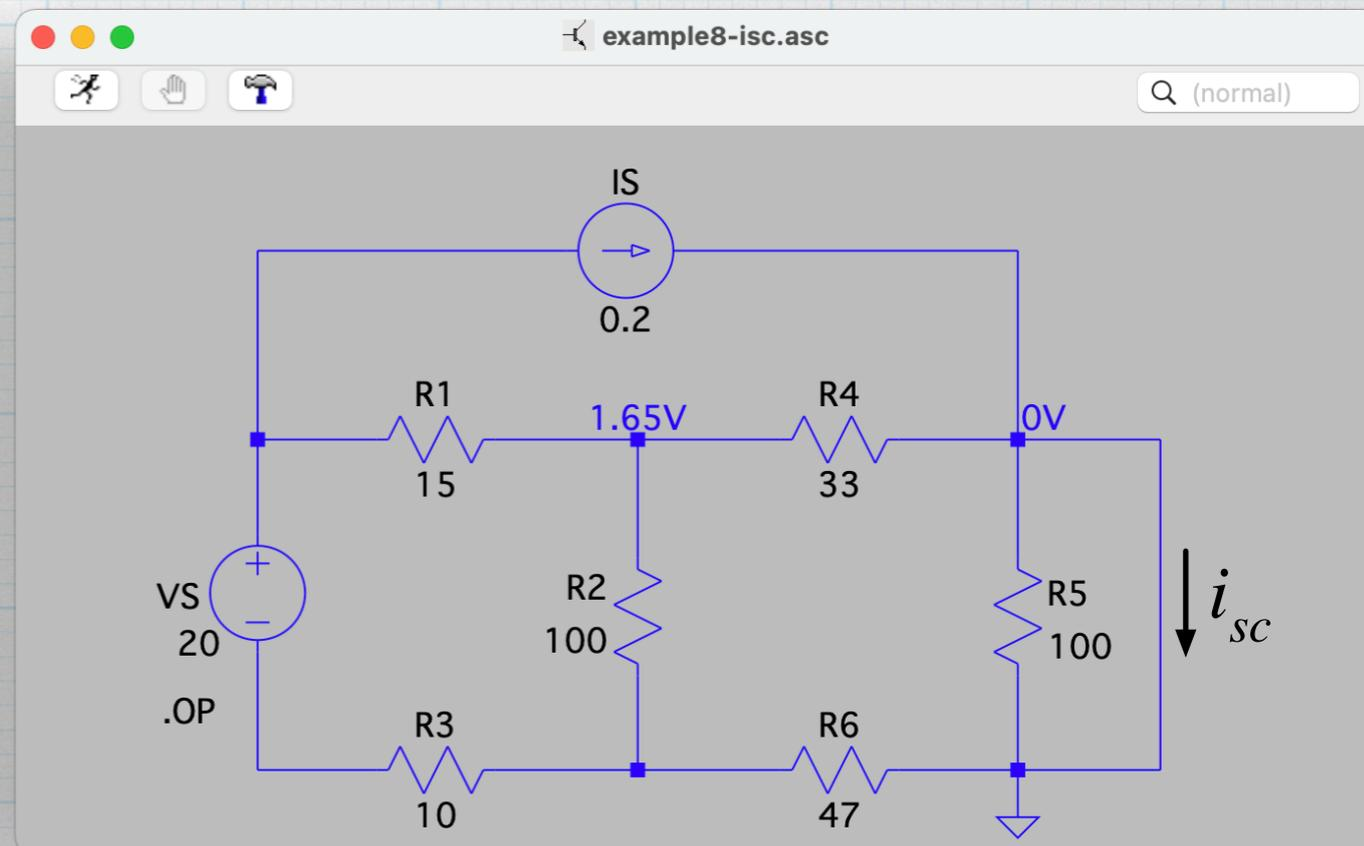
$$I_N = i_{sc} = 0.2 \text{ A} + (1.65 \text{ V}) / (33 \text{ } \Omega) = 0.25 \text{ A.}$$
