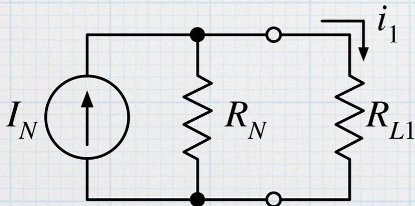
$$i_1 = \frac{\frac{1}{R_{L1}}}{\frac{1}{R_{L1}} + \frac{1}{R_N}} I_N$$
