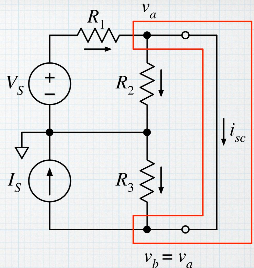
$$R_{Th} = \frac{v_{oc}}{i_{sc}} = 282 \Omega$$
