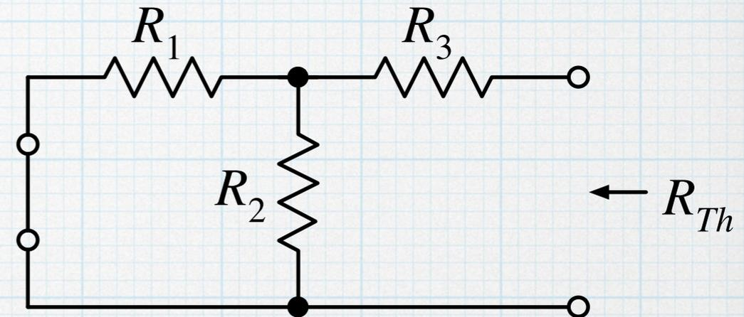
$$\begin{aligned} R_{Th} &= R_3 + R_1 \parallel R_2 \\ &= 1 \text{ k}\Omega + (2.2 \text{ k}\Omega) \parallel (3.3 \text{ k}\Omega) \\ &= 2.32 \text{ k}\Omega \end{aligned}$$
