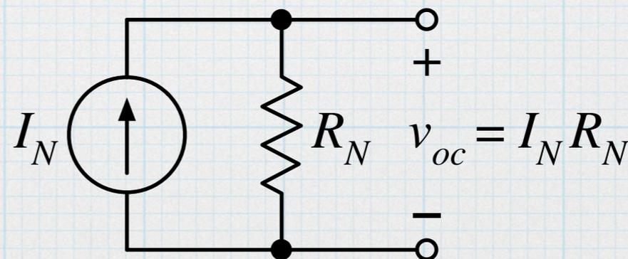
We still need a second measurement. What if we choose  $R_{L2}$  to be a short-circuit ( $R_{L2} = 0$ )? In the Norton circuit, we see that the short circuit at the load effectively shorts out  $R_N$  (no voltage across means no current through), and all of the source current must flow through the short,  $i_{sc} = I_N$ !
