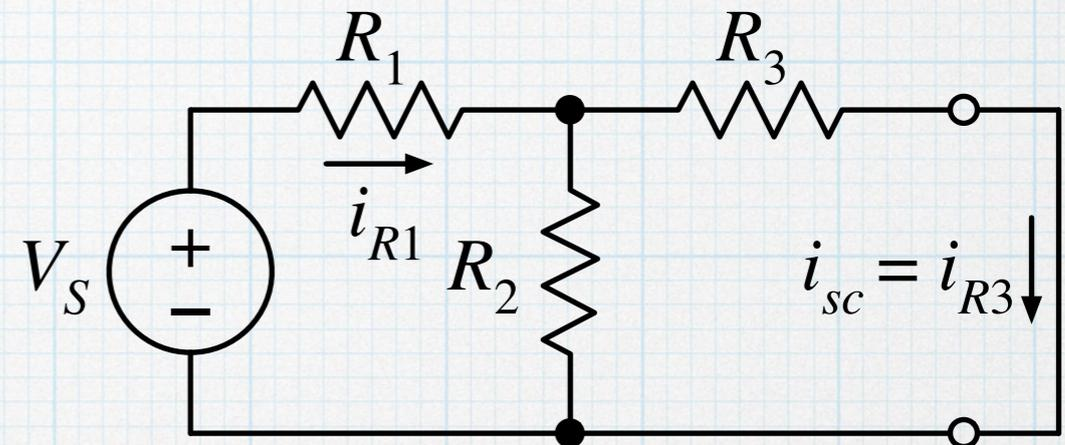
$$i_{R1} = \frac{V_S}{R_{123}} = \frac{V_S}{R_1 + R_2 \parallel R_3}$$
