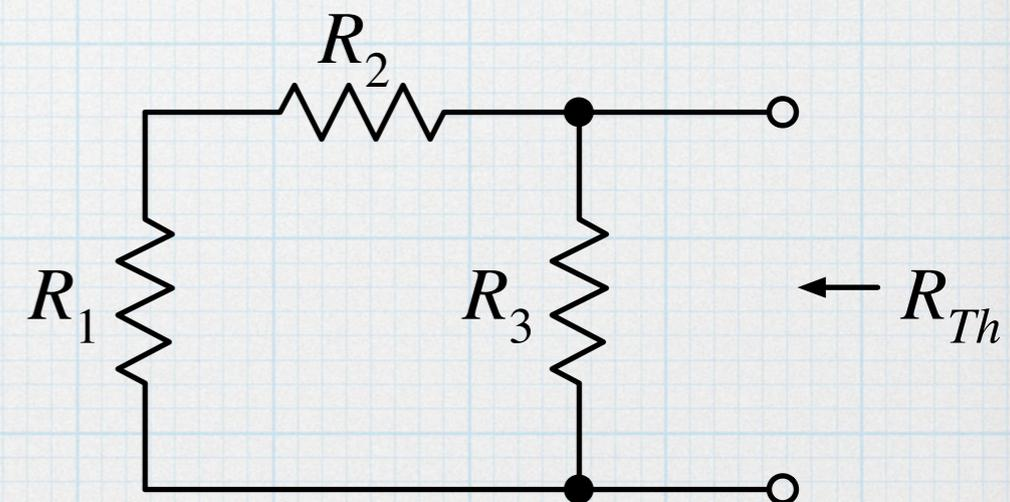
$$R_{eq} = R_{Th} = R_N = R_3 \parallel (R_1 + R_2) = 20 \Omega$$
