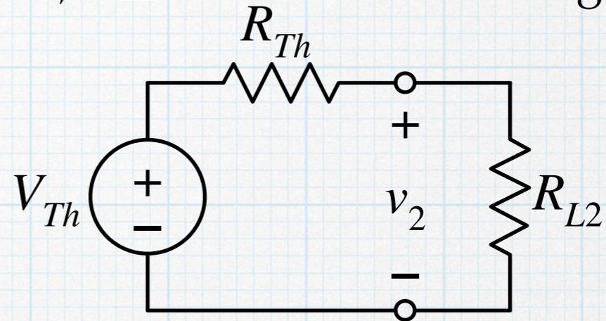
$$v_2 = \frac{R_{L2}}{R_{L2} + R_{Th}} V_{Th}$$
