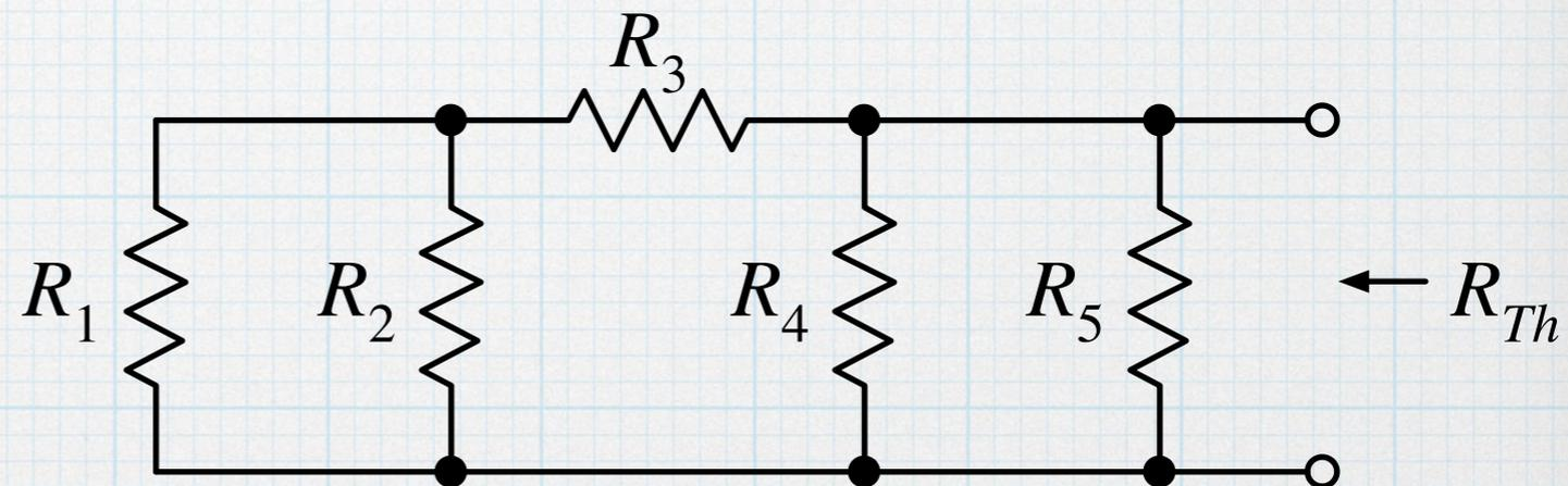
$$R_{Th} = R_5 \parallel R_4 \parallel (R_3 + R_1 \parallel R_2)$$
