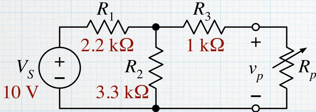
Circuit with 10-turn, 10-kΩ potentiometer as the load.
