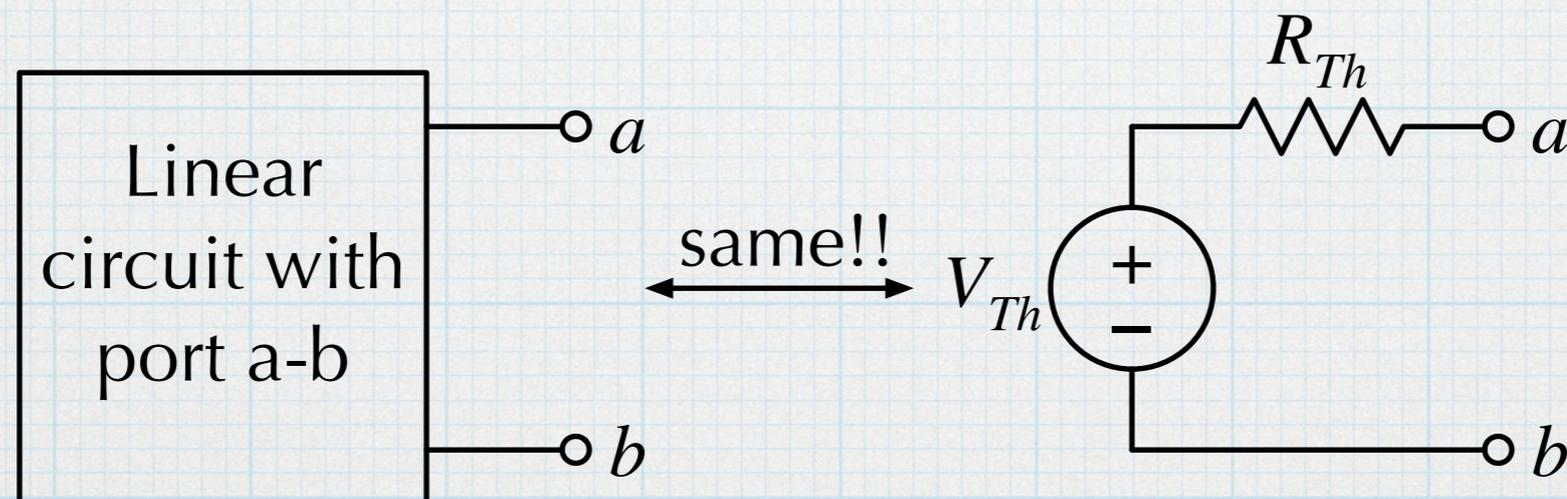
This view that every linear circuit has an effective voltage (which could be zero!) and an effective resistance completely changes the way that we look at circuits.
