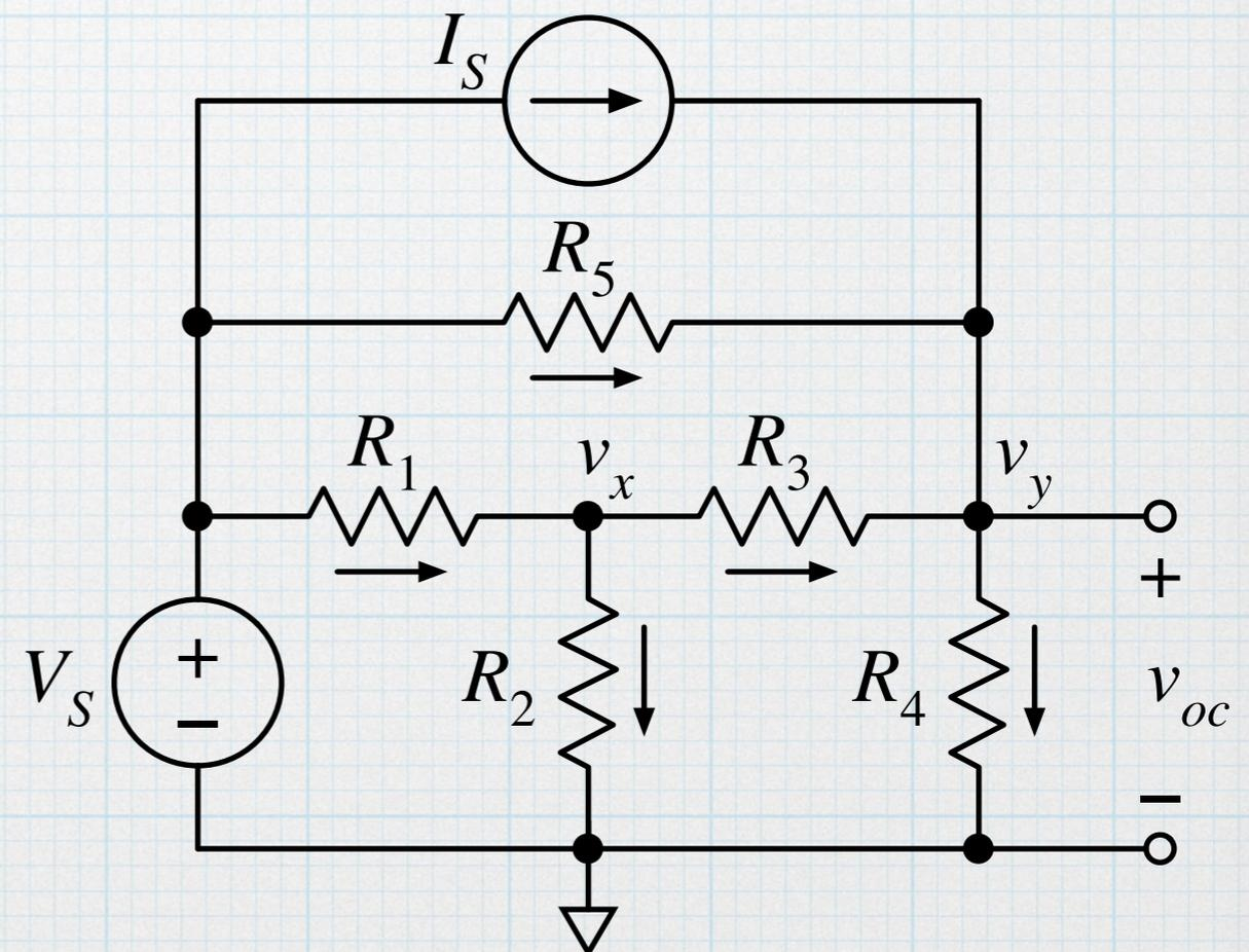
Inserting values and solving gives  $v_x = 11$  V and  $v_y = 15$  V. So  $V_{Th} = 15$  V.
