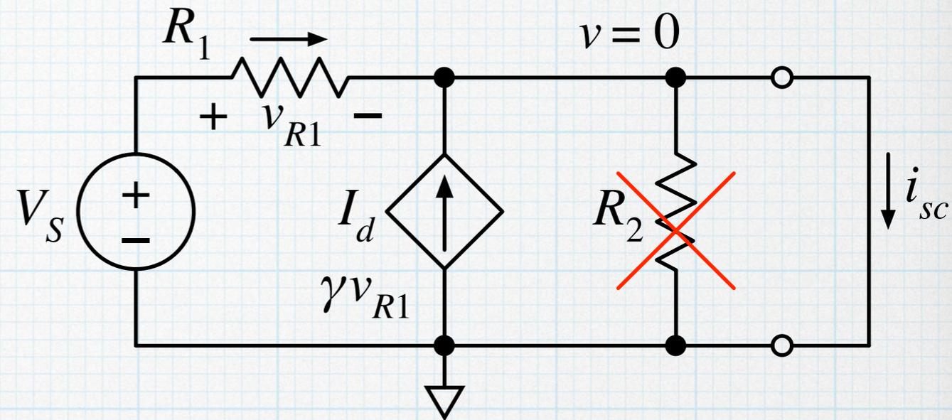
Note that if we had incorrectly tried to use the short-cut method for finding  $R_{Th}$ , we would have shorted the voltage source and then probably removed the dependent current source, leaving the two resistors in parallel. The result would have been “close-ish” to the actual value, but definitely not correct.
