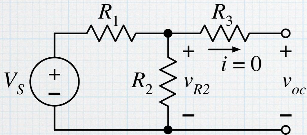
$$v_{oc} = v_{R2} = \frac{R_2}{R_1 + R_2} V_S$$
