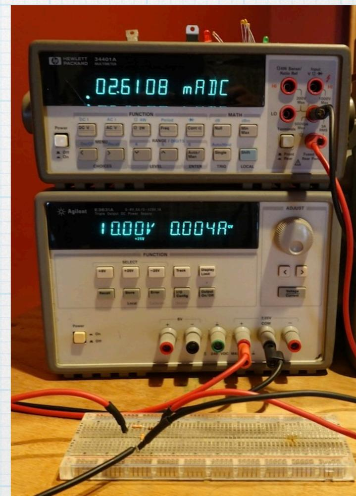
$$R_{Th} = \frac{6 \text{ V}}{2.61 \text{ mA}} = 2.30 \text{ k}\Omega$$
