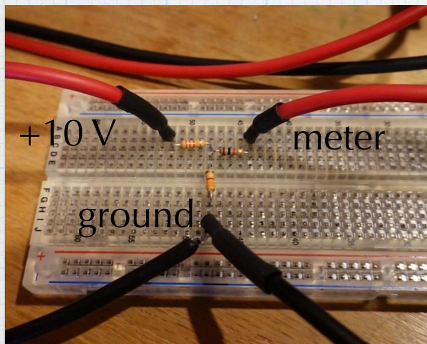
$$v_{oc} = 6 \text{ V} = V_{TH}$$
