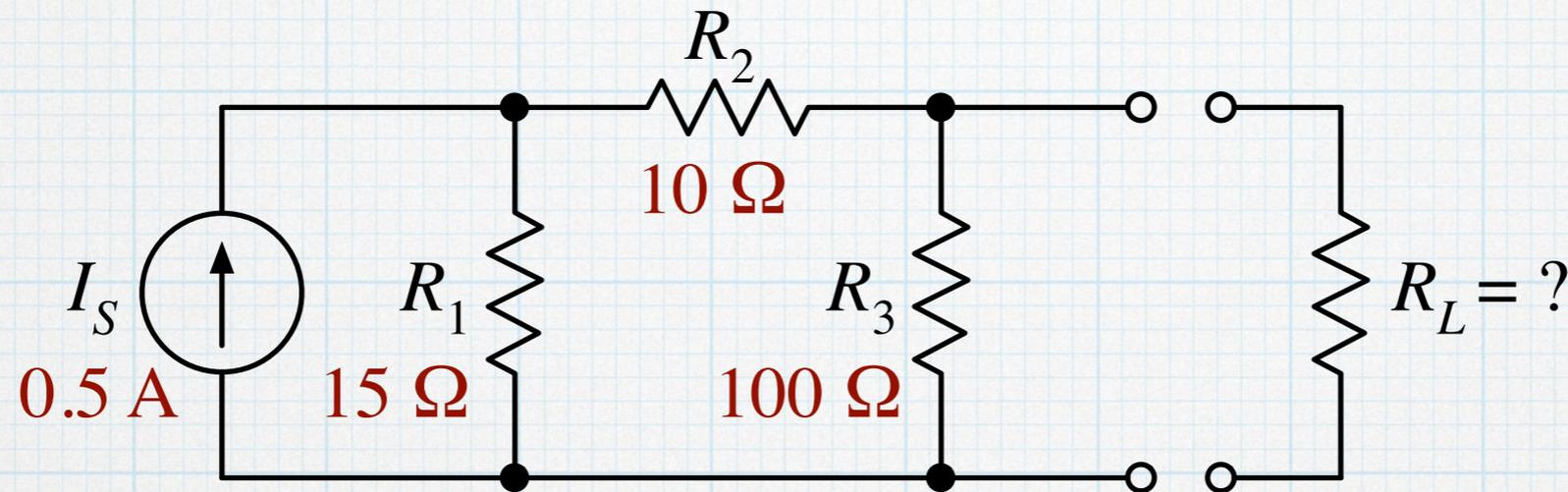
This is a Thevenin/Norton equivalent problem in disguise. Obviously, we need to find an equivalent circuit. We can start by finding the resistance. Since there is only a single independent source, we can use the short-cut method. After deactivating  $I_S$ :
