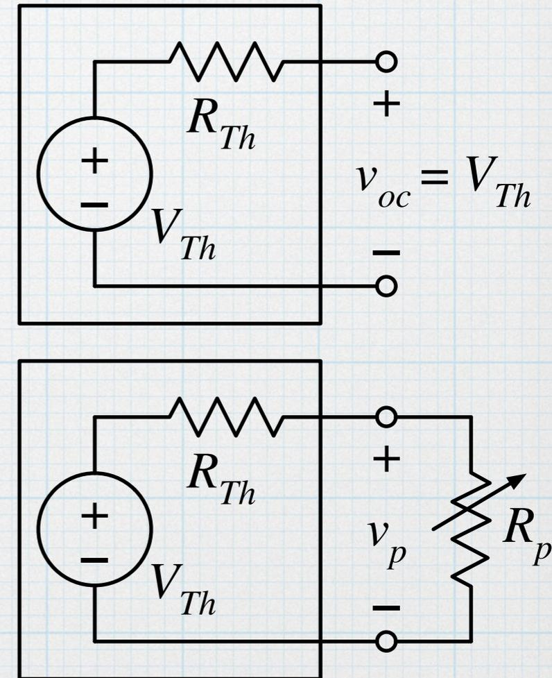
$$v_p = \frac{v_{oc}}{2} \text{ when } R_p = R_{Th}.$$
