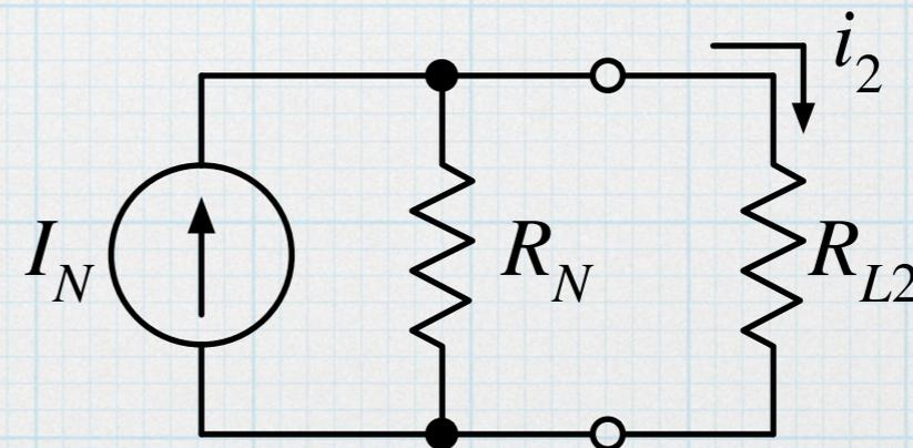
$$i_2 = \frac{\frac{1}{R_{L2}}}{\frac{1}{R_{L2}} + \frac{1}{R_N}} I_N$$
