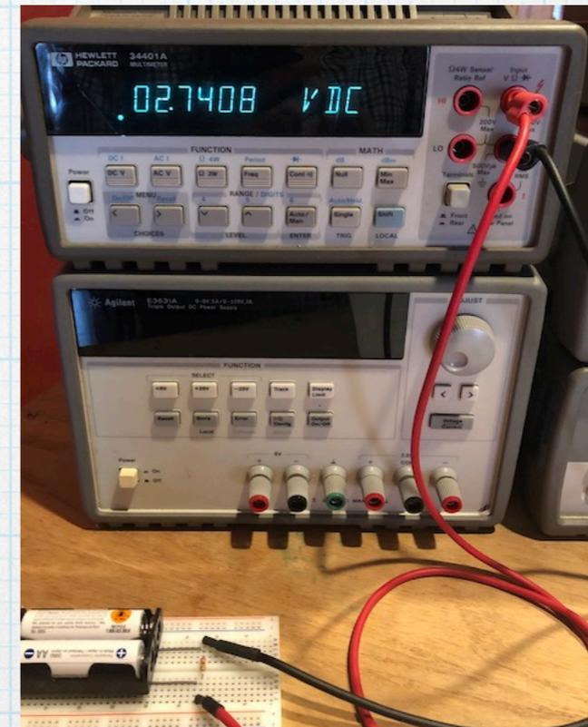
$$V_{Th} = \frac{v_1 v_2 (R_{L1} - R_{L2})}{R_{L1} v_2 - R_{L2} v_1} = 2.87 \text{ V} \quad \text{and} \quad R_{Th} = \frac{R_{L1} R_{L2} (v_1 - v_2)}{R_{L1} v_2 - R_{L2} v_1} = 1.03 \Omega.$$
