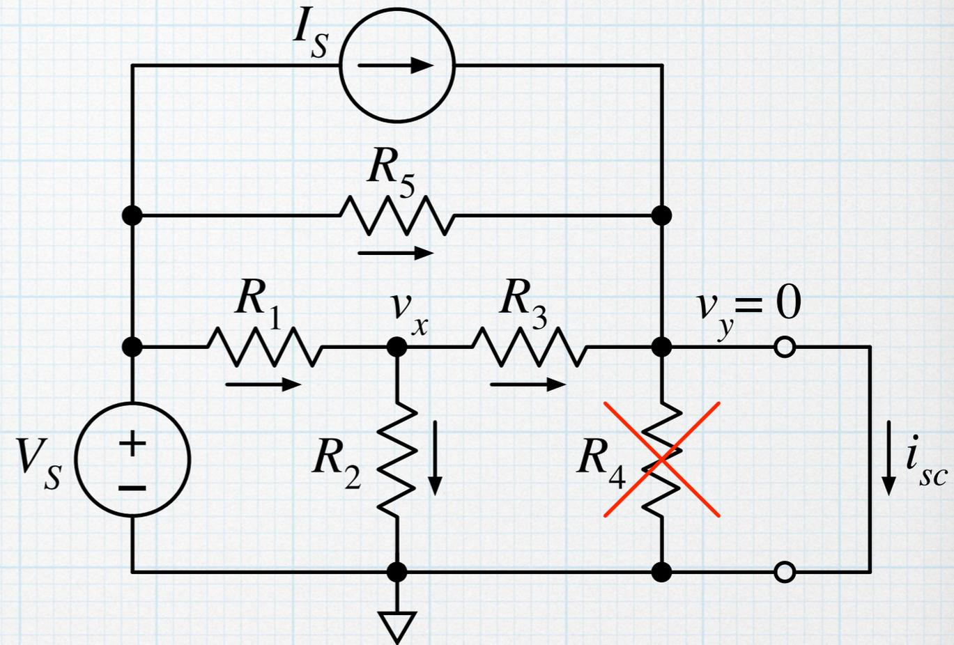
To find  $i_{R3}$ , we will need to determine the node voltage,  $v_x$ . Writing the NV equation:
