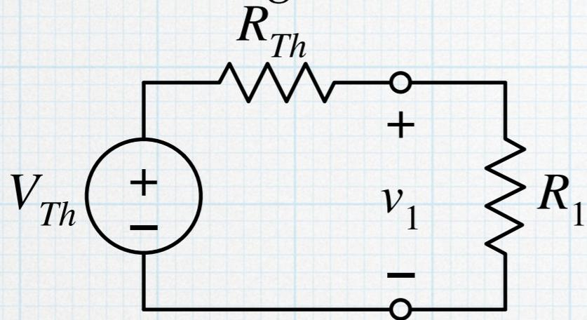
$$v_1 = \frac{R_{L1}}{R_{L1} + R_{Th}} V_{Th}$$
