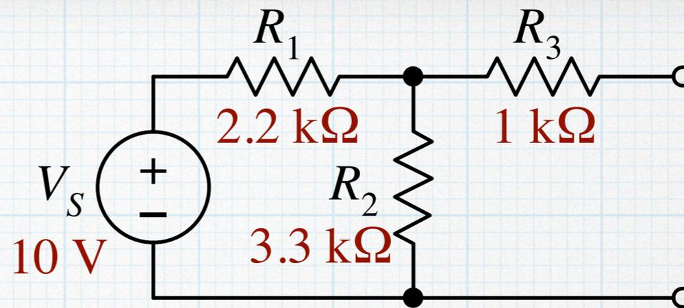
First, do the measurement in the lab. It's easy — just build the circuit on a breadboard with the 10-V supply for  $V_S$ . Use the multimeter at the port to first measure  $v_{oc}$  and then switch over to measure  $i_{sc}$ .
