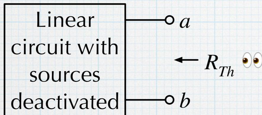
This works because the equivalent resistance derives from the network of resistors in the original circuit. If we remove the sources (deactivate them), we are left with just resistors, allowing us to find the equivalent resistance using the resistor reduction techniques learned earlier.
