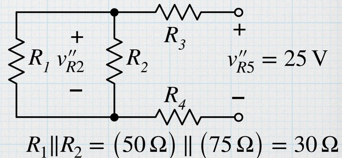
Finally,  $I_S$ . Deactivate  $V_{S1}$  and  $V_{S2}$  in the original circuit. The source current divides to the left and right according to the equivalent resistances on either side. First find the equivalent resistances left and right:
