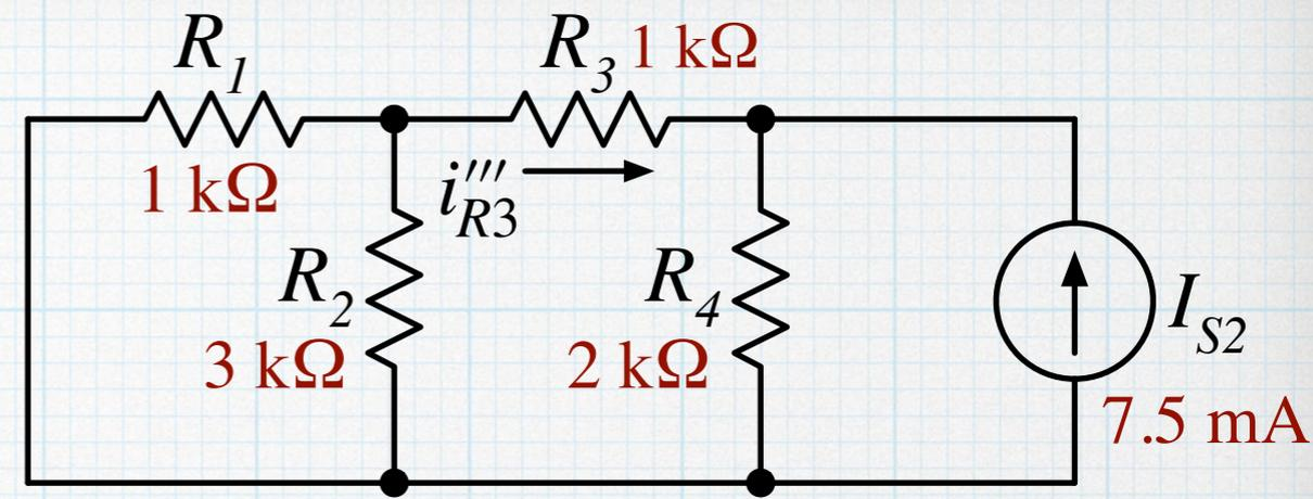
Again, we can find the current with a current divider. The source current splits between two paths – the branch with  $R_4$  and another that is a combination of  $R_1$ ,  $R_2$ , and  $R_3$ . Also, note carefully the direction –  $i'''_{R3}$  will be negative!
