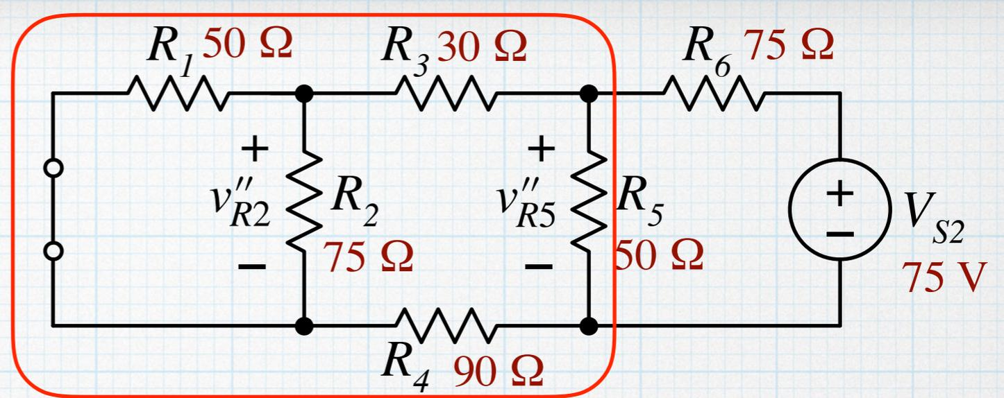
Use voltage dividers twice: first to find the voltage across  $R_5$ , then again to find voltage across  $R_2$ . Need the equivalent resistance of  $R_5$  and all of the stuff in parallel with it, seen looking back from  $V_{S2}$ .
