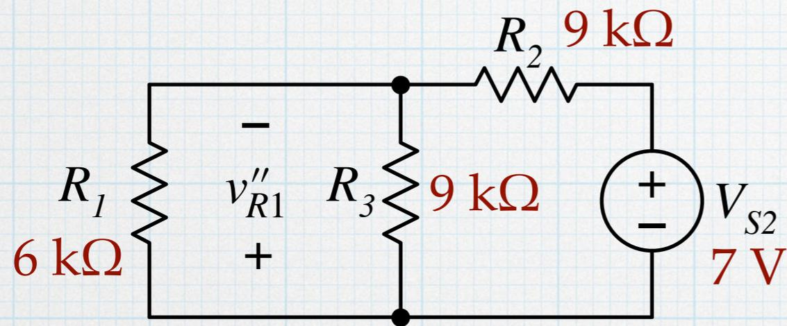
$$v''_{R1} = - \frac{R_1 \parallel R_3}{R_1 \parallel R_3 + R_2} V_{S2}$$
