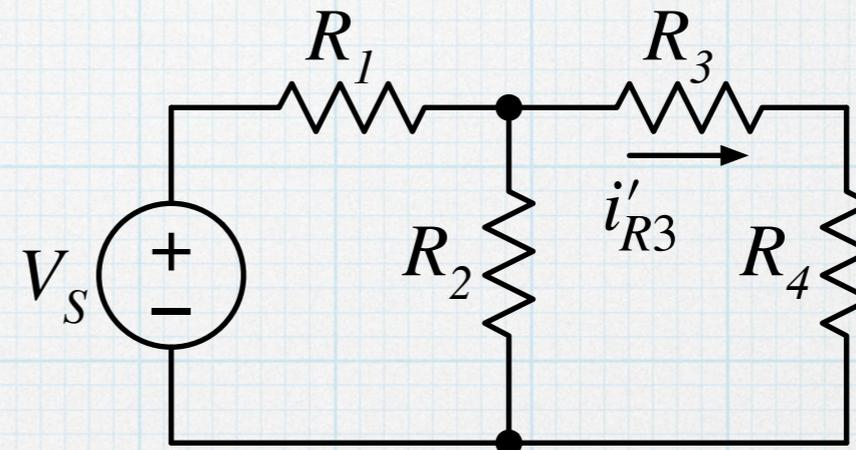
$$I'_S = \frac{V_S}{R_1} = \frac{10 \text{ V}}{1 \text{ k}\Omega} = 10 \text{ mA}$$
