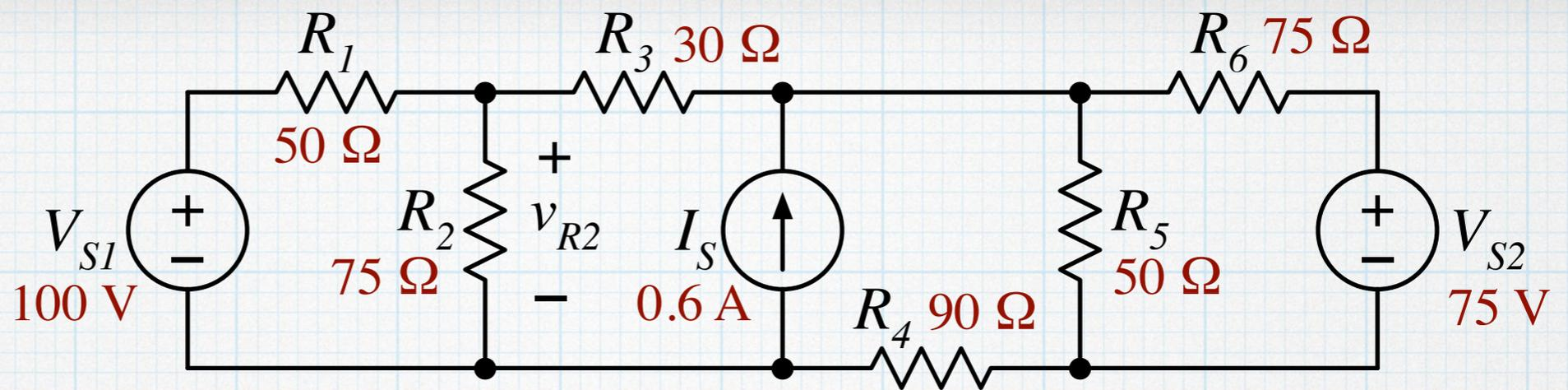
This looks nasty – there are 6 nodes with a super node or 4 meshes with a super mesh. Either NV or MC will be tough. We might be able to do a bunch of source transformations, but since there are only three sources, let's try superposition.
