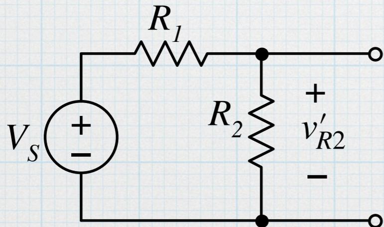
$$\begin{aligned} v'_{R2} &= \frac{R_2}{R_1 + R_2} V_S \\ &= \frac{5 \Omega}{5 \Omega + 10 \Omega} (10 \text{ V}) = 3.33 \text{ V} \end{aligned}$$
