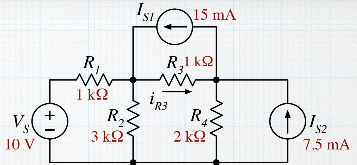
1. Start with  $V_S$ . Deactivate the two current sources. Find the partial current, using whatever short-cut methods you like. One approach: use a source transformation and then a current divider.
