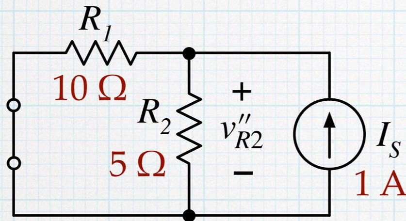
Shorting  $V_S$  causes  $R_1$  to be in parallel with  $R_2$ .
