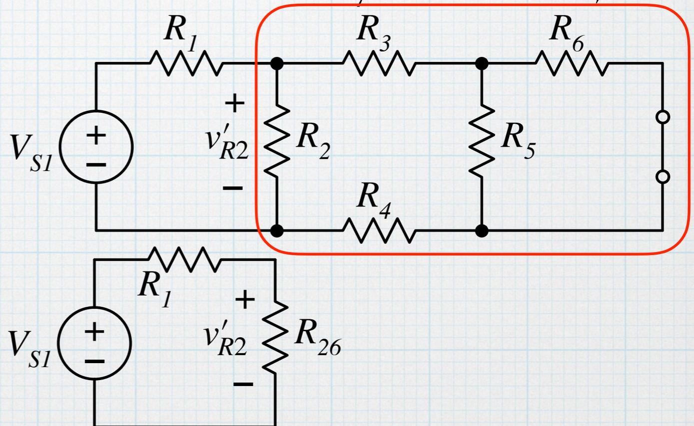
$$R_{26} = R_2 \parallel (R_3 + R_4 + R_5 \parallel R_6) = (75 \Omega) \parallel [30 \Omega + 90 \Omega + (50 \Omega) \parallel (75 \Omega)] = 50 \Omega$$
