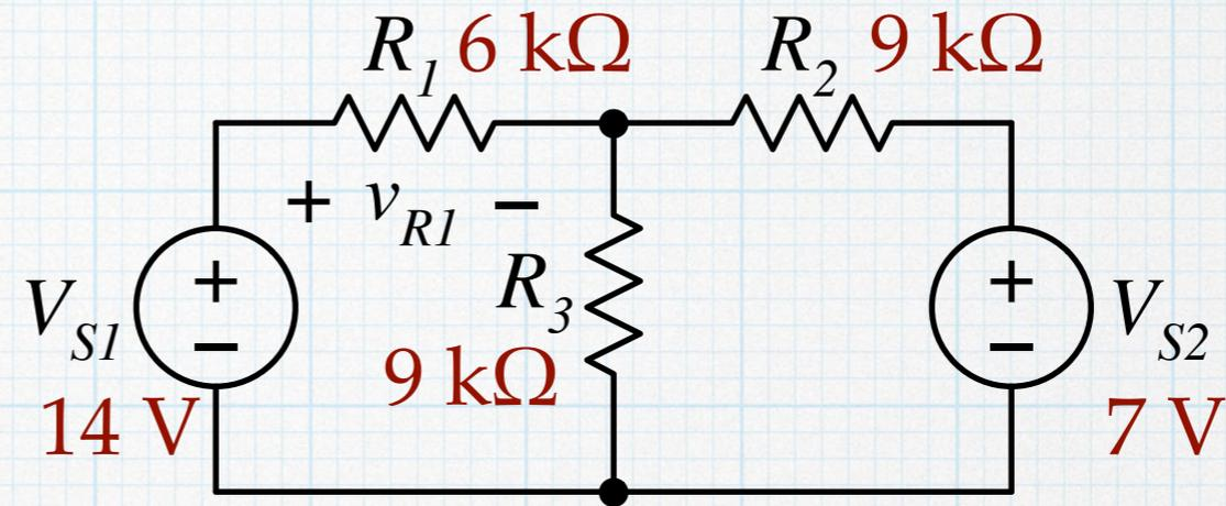
1. Deactivate  $V_{S2}$ . The result is a voltage divider between  $R_1$  and the parallel combination of  $R_2$  and  $R_3$ .
