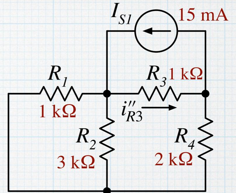
$$R_{124} = R_1 \parallel R_2 + R_4 = 1 \text{ k}\Omega \parallel 3 \text{ k}\Omega + 2 \text{ k}\Omega = 2.75 \text{ k}\Omega$$
