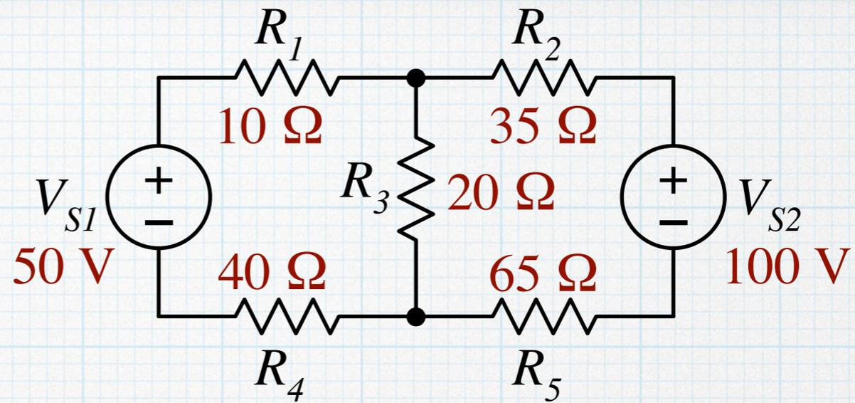
1. In using superposition, we cannot find “partial powers” — we need to find either total voltage or total current and then calculate power. For this problem, we will choose to find  $v_{R3}$ . Start by deactivating  $V_{S2}$ . We note that the series combination of  $R_2$  and  $R_5$  is in parallel with  $R_3$ .
