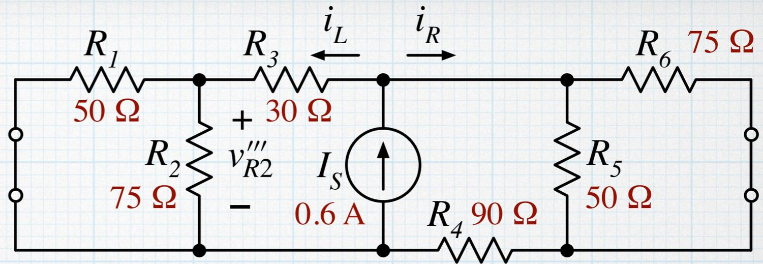
$$R_L = R_3 + R_1 \parallel R_2$$
