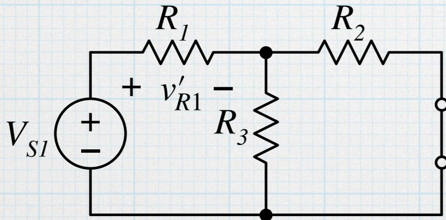
$$\begin{aligned} v'_{R1} &= \frac{R_1}{R_1 + R_2 \parallel R_3} V_{S1} \\ &= \frac{6 \text{ k}\Omega}{6 \text{ k}\Omega + (9 \text{ k}\Omega \parallel 9 \text{ k}\Omega)} (14 \text{ V}) = 8 \text{ V} \end{aligned}$$
