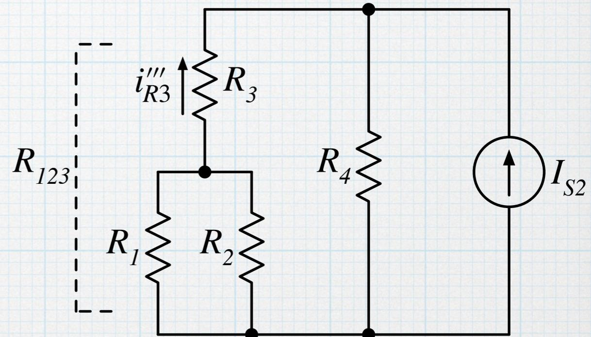
$$R_{123} = R_1 \parallel R_2 + R_3 = 1 \text{ k}\Omega \parallel 3 \text{ k}\Omega + 1 \text{ k}\Omega = 1.75 \text{ k}\Omega$$
