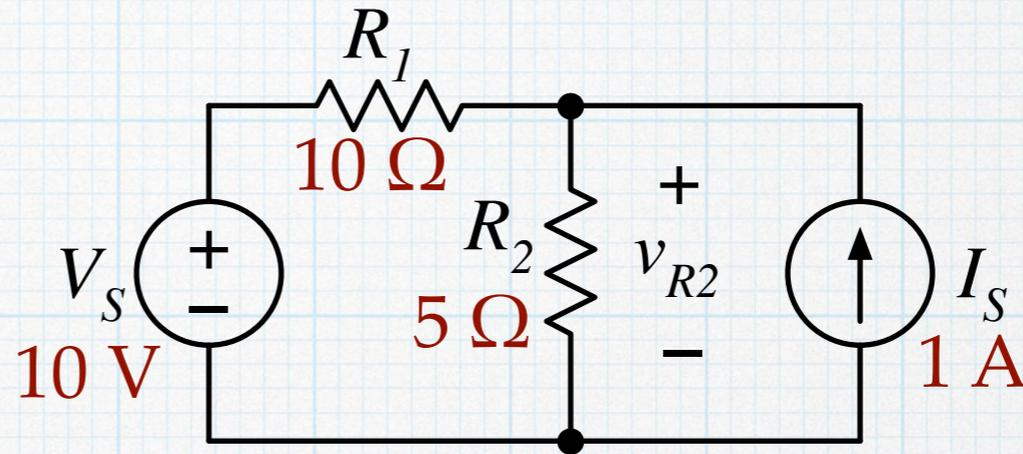
1. Deactivate (turn off) one of the sources — the order doesn't matter. Let's deactivate the current source first — set the value of  $I_S$  to zero, which has the same effect as replacing  $I_S$  with an open circuit. The result is a simple voltage divider, and we can easily calculate the partial result due to the voltage source.
