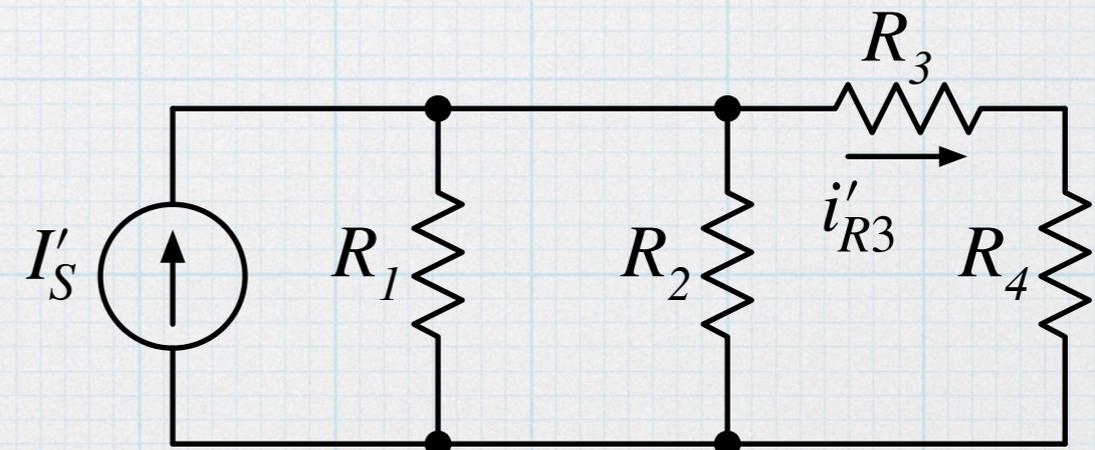
$$i'_{R3} = \frac{\frac{1}{R_3 + R_4}}{\frac{1}{R_3 + R_4} + \frac{1}{R_1} + \frac{1}{R_2}} I'_S = \frac{\frac{1}{3 \text{ k}\Omega}}{\frac{1}{3 \text{ k}\Omega} + \frac{1}{1 \text{ k}\Omega} + \frac{1}{3 \text{ k}\Omega}} (10 \text{ mA}) = 2 \text{ mA}$$
