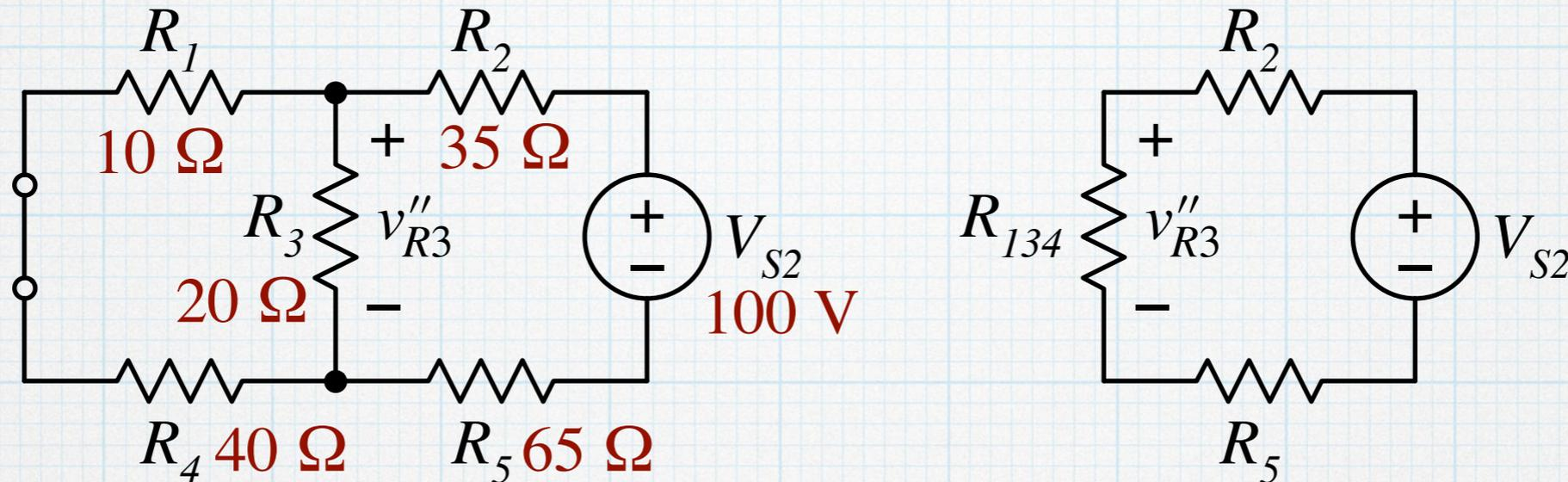
$$R_{134} = R_3 \parallel (R_1 + R_4)$$
