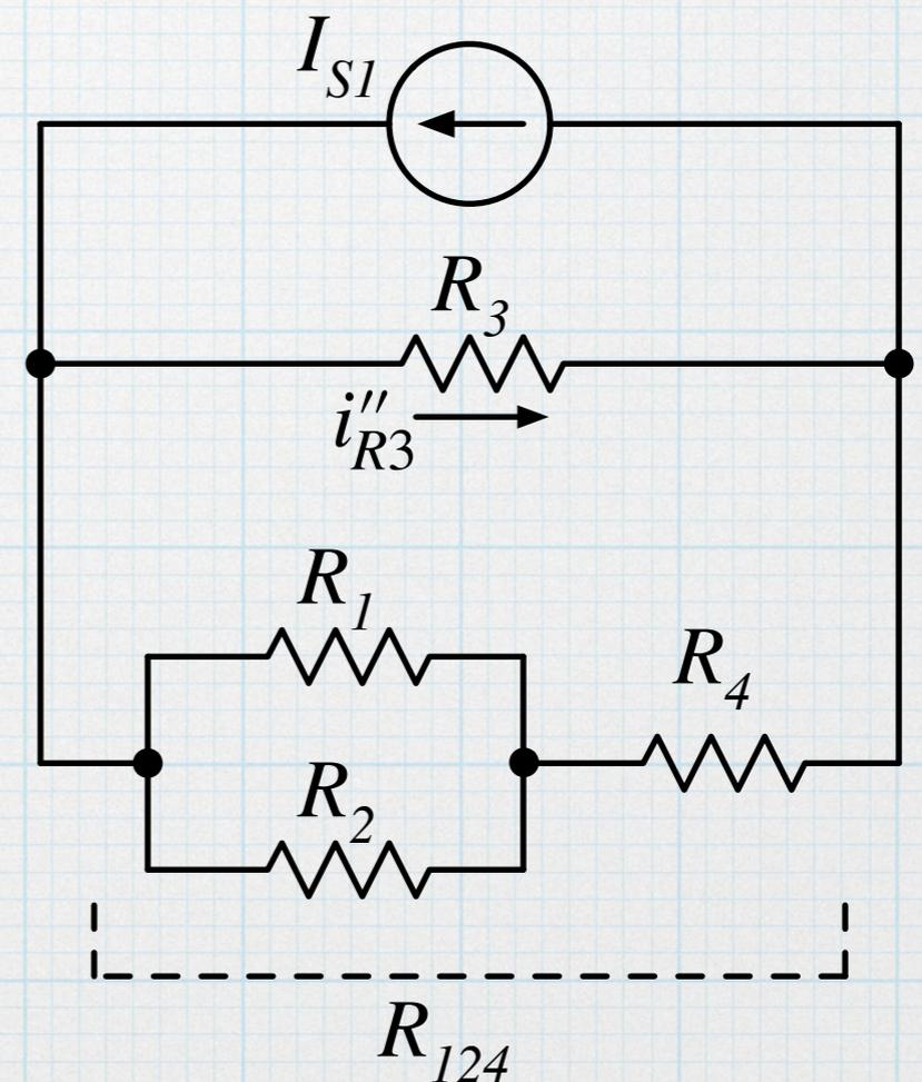
3. To obtain the final partial circuit, go back to the original circuit and deactivate  $V_S$  and  $I_{S1}$ , keeping  $I_{S2}$ . As in the prior case,  $R_1$  is in parallel with  $R_2$ .
