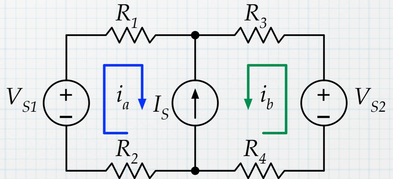
Define the voltages for the components around each mesh and write KVL equations.
