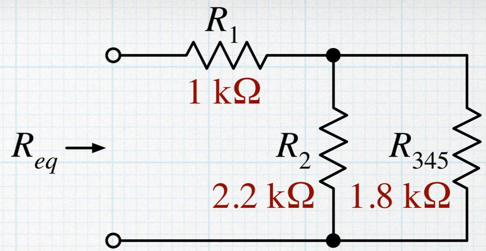
Calculate the equivalent resistance of the parallel combination. Using the two-resistor formula:
