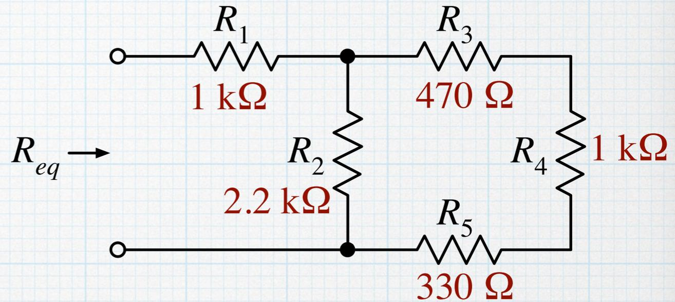
The trick is to break the circuit into smaller pieces that are purely series or parallel, find the equivalent of that piece and insert that back into the original circuit, which will now be simpler. Then find another series or parallel combination that can be simplified. Through a sequence of steps, it may be possible to reduce even complex combinations to a single equivalent resistance.
