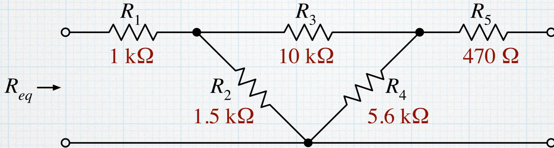
There are a couple of interesting things going on here. First, we see some “diagonal” resistors. Secondly, we see a “dangling” resistor,  $R_5$ , which is not connected to anything on one side.
