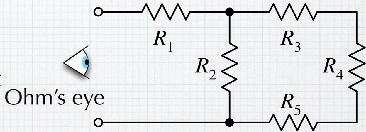
2. Starting at the opposite end of the network, identify series and parallel combinations that can be reduced using the simple formulas.
