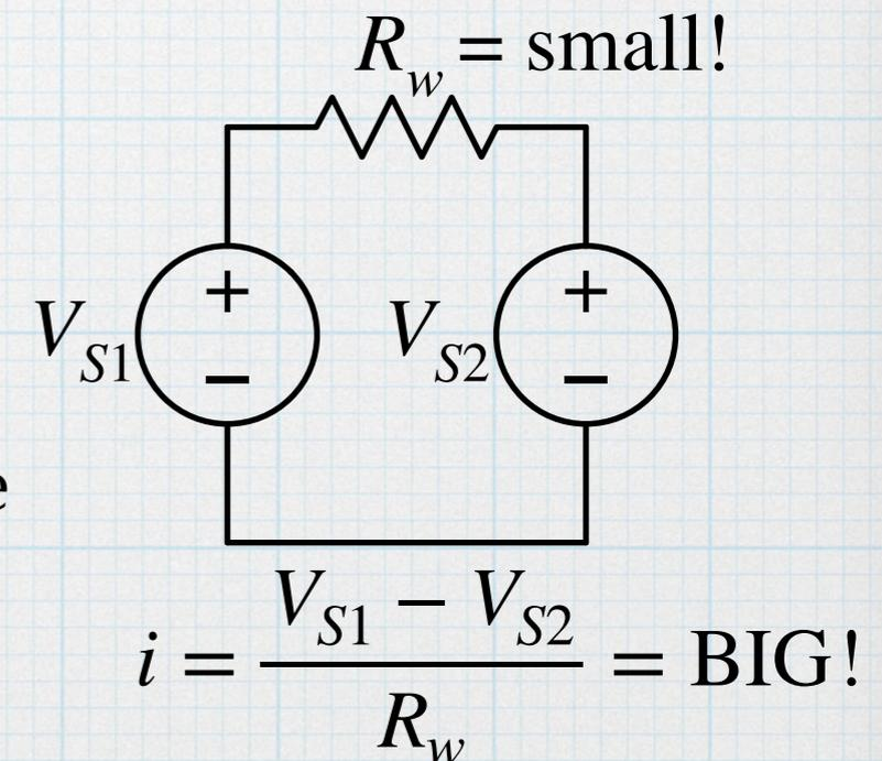
If we connect two random batteries together (or short out a battery —  $V_{S2} = 0$ ), bad things may happen. A practical battery charger will have some means to limit current. In fact, it may actually be current source.
