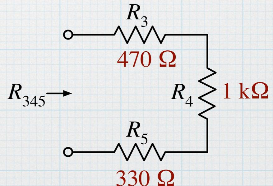
Insert the single  $R_{345}$  resistor back into the original circuit. Now, quite obviously,  $R_2$  is in parallel with  $R_{345}$ .
