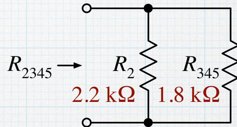
$$R_{2345} = \frac{R_2 \cdot R_{345}}{R_2 + R_{345}} = \frac{(2.2 \text{ k}\Omega) (1.8 \text{ k}\Omega)}{(2.2 \text{ k}\Omega) + (1.8 \text{ k}\Omega)} = 990 \Omega$$
