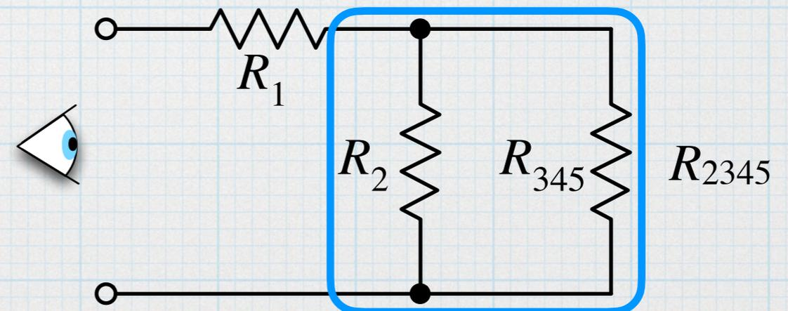
4. Continue the simplification process, one series or parallel combination at a time, until the network is reduced to a single resistor. (Or until the remaining network is trivial.)
