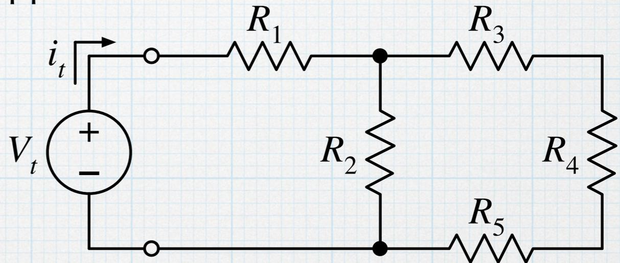
In lab we could do something similar by building the circuit, applying a test voltage, and measuring the resulting current. In lab, this process goes by a different name — it’s called “using an ohmmeter”.
