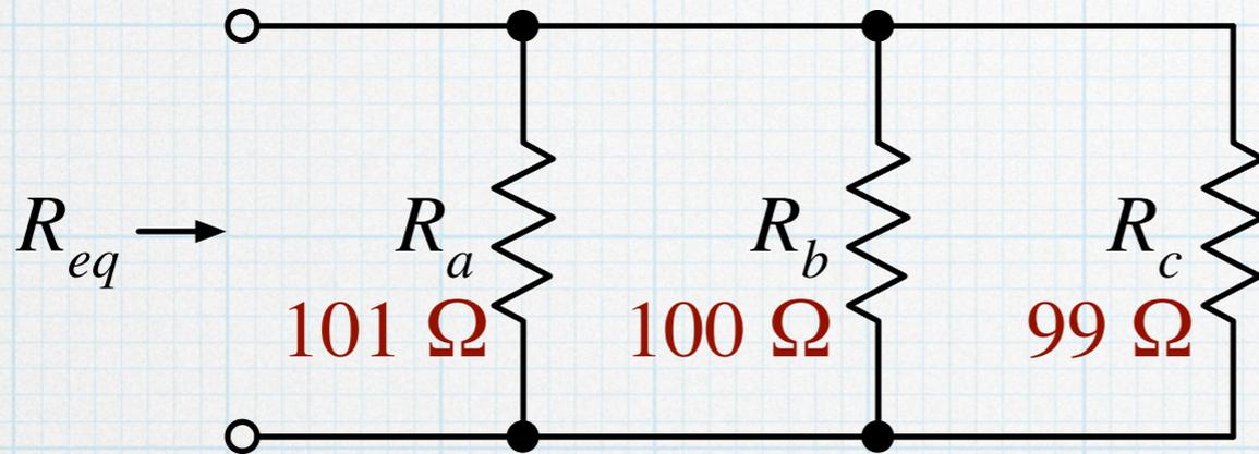
$$R_{eq} = \frac{1}{\frac{1}{R_a} + \frac{1}{R_b} + \frac{1}{R_c}} = 33.3 \Omega$$
