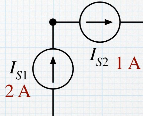
KCL:  $I_{S1} \neq I_{S2} : \text{In} \neq \text{Out}!!$  Yikes!
