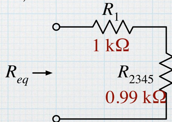
$$R_{eq} = R_1 + R_{2345} = 1 \text{ k}\Omega + 0.99 \text{ k}\Omega = 1.99 \text{ k}\Omega.$$
