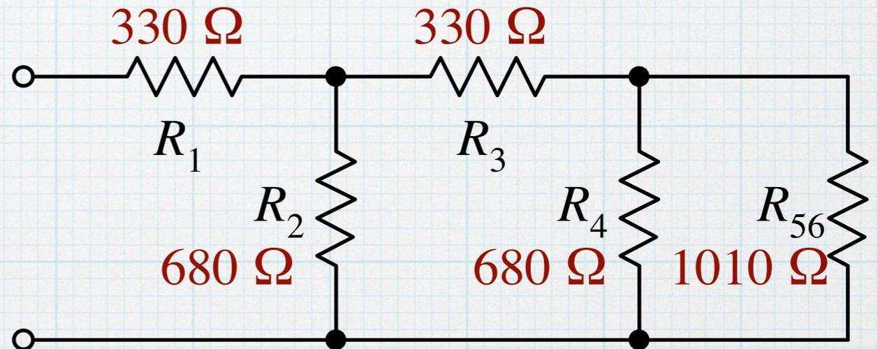
2.  $R_4$  is in parallel with  $R_{56}$ .
