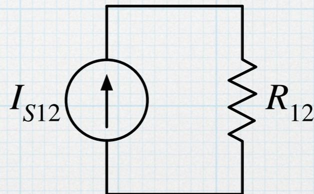
All the components have the same voltage across,  $v_{I_{S1}} = v_{I_{S2}} = v_{R1} = v_{R2} = v_S$ . We know that we can combine the parallel resistors, and it appears that we can combine the current sources as well.
