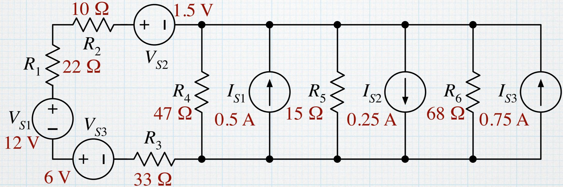
Three resistors in series on the left:  $R_L = R_1 + R_2 + R_3 = 65\ \Omega$
