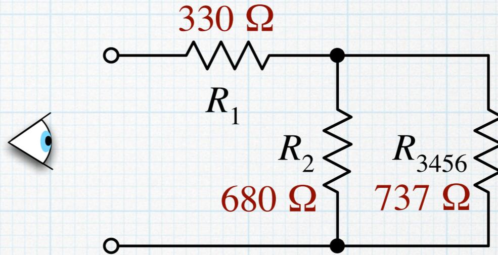
4.  $R_2$  is in parallel with  $R_{3456}$ .
