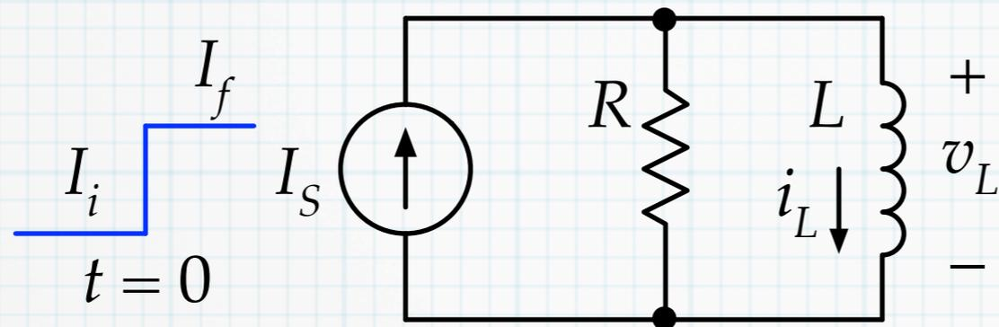
In the circuit,  $I_S$  abruptly changes value from  $I_i$  to  $I_f$  at  $t = 0$ . Assume that the source was at  $I_i$  for a “very long time” before  $t = 0$ .
