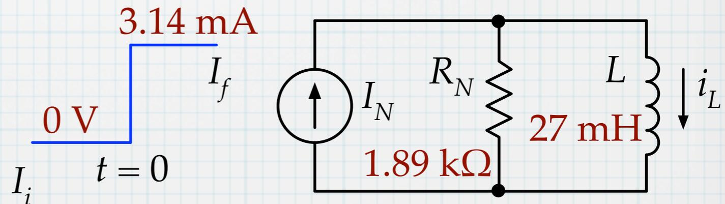
$$i_L(t) = [3.14 \text{ mA}] \left[ 1 - \exp\left(-\frac{t}{14.3 \text{ }\mu\text{s}}\right) \right]$$
