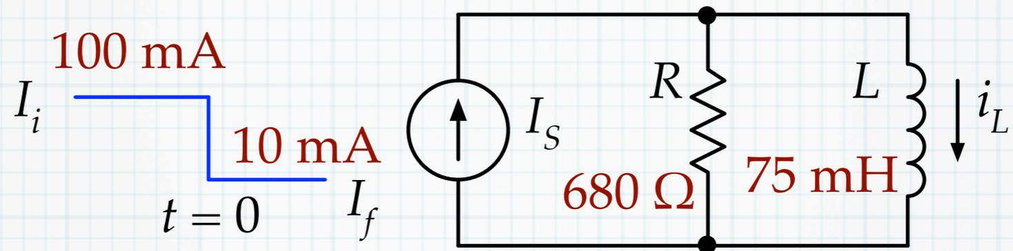
In the  $RL$  circuit above,  $I_s$  abruptly changes value from  $I_i = 100 \text{ mA}$  to  $I_f = 10 \text{ mA}$  at  $t = 0$ . Assume that the source was at  $I_i$  for a “very long time” before  $t = 0$ . Find the expression for the inductor current as a function of time. Find the time at which  $i_L = 50 \text{ mA}$ .
