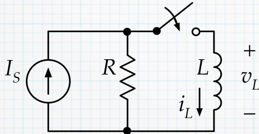
1. For  $t < 0$ , the inductor may have a current flowing (depending on the circuit configuration),  $i_L(t < 0) = I_i$ . Also,  $v_L = 0$ .
