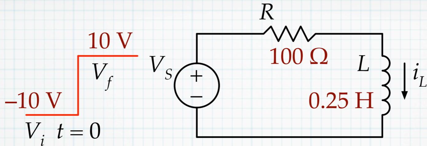
The voltage source in the above circuit abruptly changes from  $-10\text{ V}$  to  $+10\text{ V}$  at  $t = 0$ . Find expressions for the inductor current and inductor voltage. Find the time at which the inductor current crosses  $0\text{ mA}$ .
