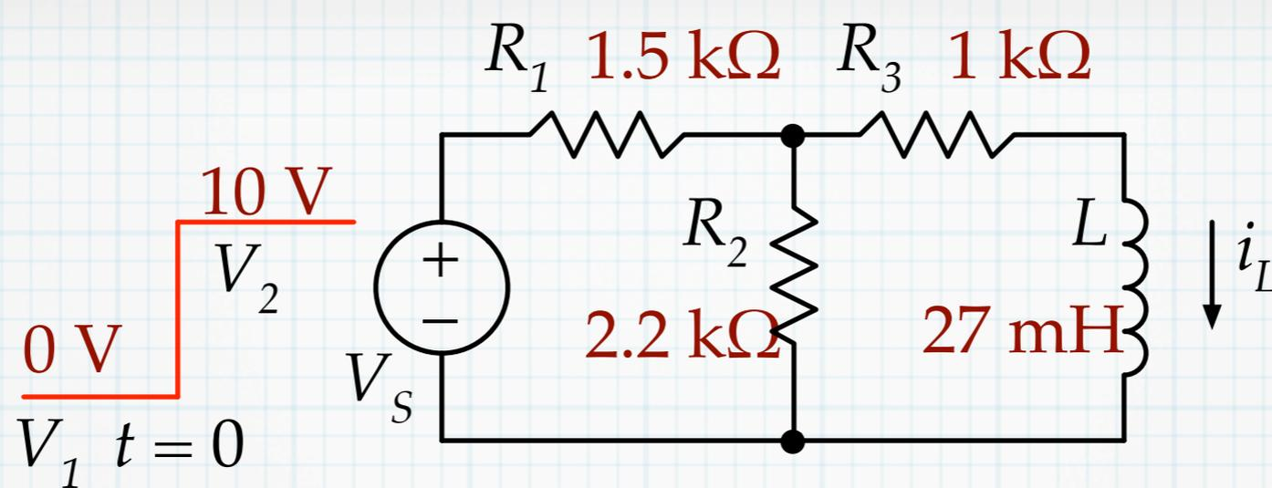
In the  $RL$  circuit above,  $V_S$  abruptly changes value from  $V_1$  to  $V_2$  at  $t = 0$ . Find the expression for the inductor current as a function of time.
