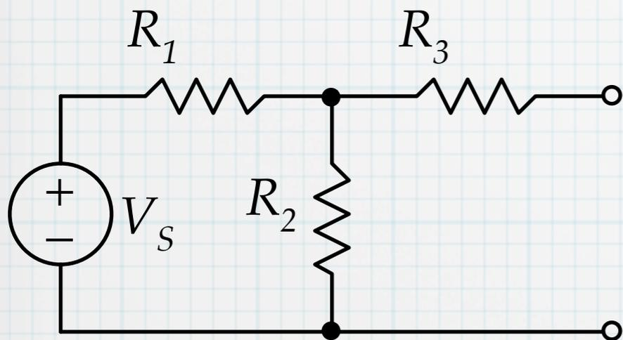
$$I_N = \frac{V_S}{R_1 + \left(1 + \frac{R_1}{R_2}\right) R_3} = 0.314 V_S.$$
