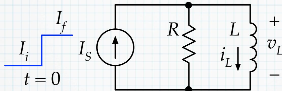
In the circuit,  $I_S$  abruptly changes value from  $I_i$  to  $I_f$  at  $t = 0$ . Assume that the source was at  $I_i$  for a “very long time” before  $t = 0$ .
