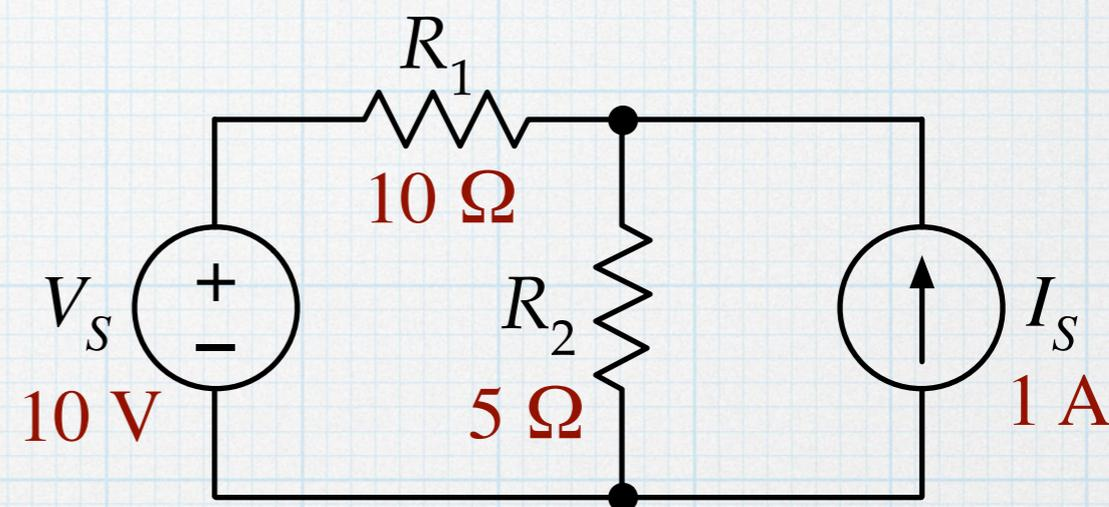
$$v_b = \frac{10 \text{ V} + (1 \text{ A})(10 \Omega)}{1 + \frac{10 \Omega}{5 \Omega}}$$
