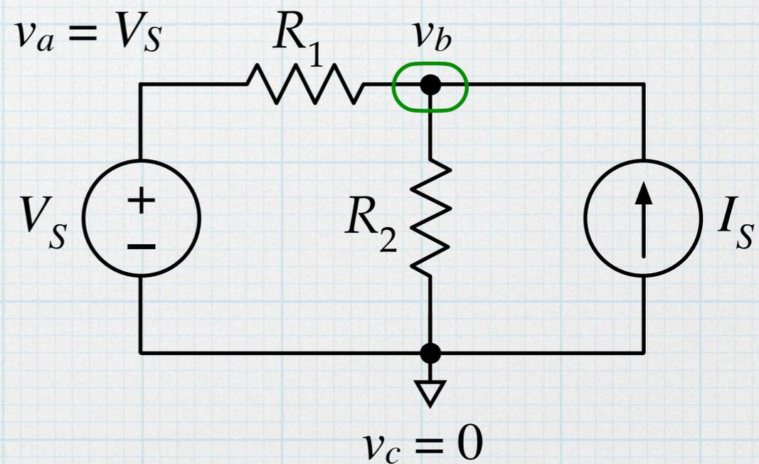
**Step 6** – Assign currents to all of the branches connected to the nodes. In principle, the direction is arbitrary. Label the voltage polarity for any resistors. (Be sure to get the polarities correct!)
