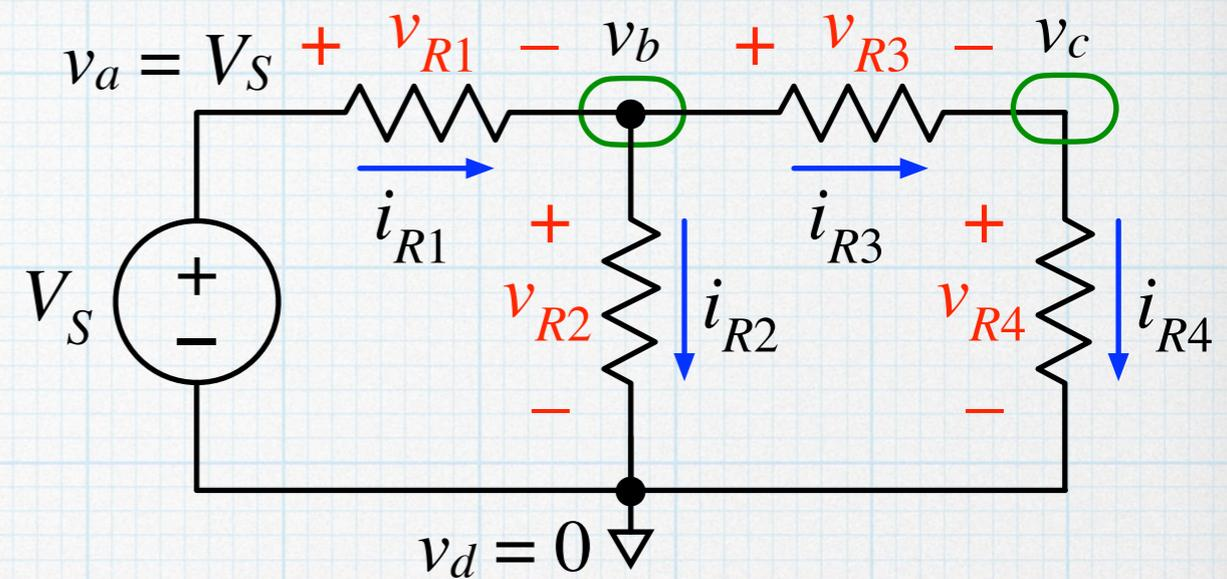
**Step 7** – Write KCL equations relating the currents at each of the unknown nodes.
