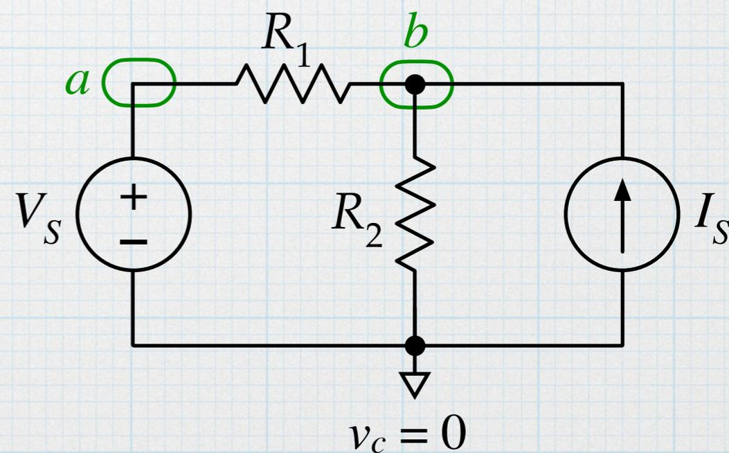
**Step 3** – Identify other nodes for which the voltage is known. In this case, the source  $V_S$  between ground and node  $a$  means that  $v_a = V_S$ .
