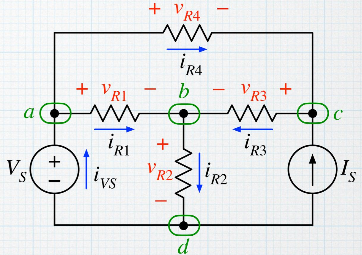
This doesn't improve the situation — there are still four equations relating five unknowns — four resistor voltages and the current flowing through the voltage source.
