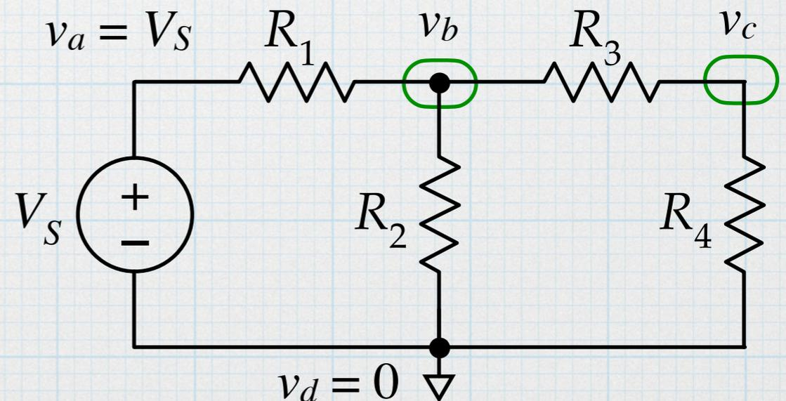
**Step 6** – Assign currents to all of the branches connected to the nodes. In principle, the direction is arbitrary. Label the voltage polarity for any resistors — take care to match voltage polarity to current direction.
