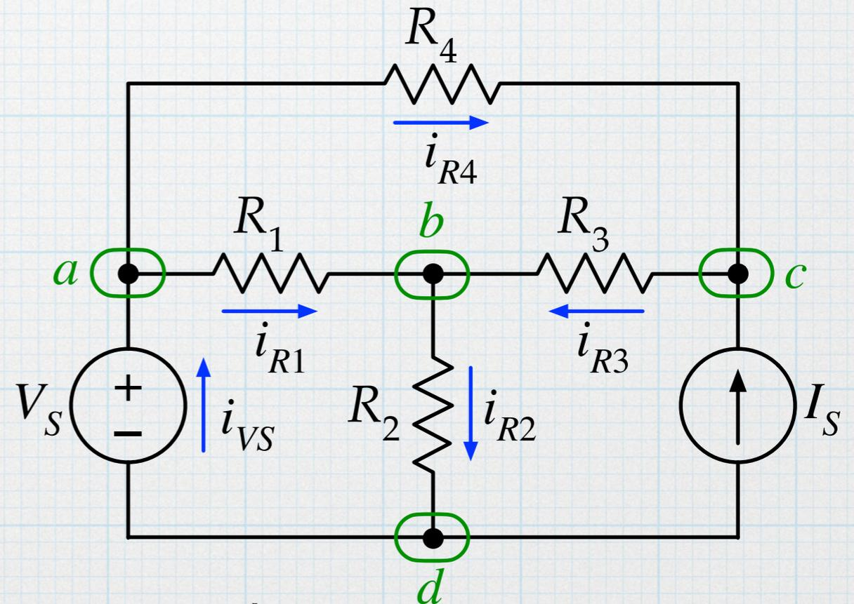
We can use Ohm's law to write resistor currents in terms of the resistor voltages. (Pay attention to polarities. For the resistors, the voltage polarities must match the chosen current directions.)
