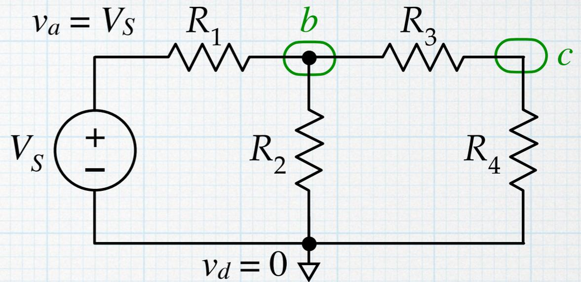
**Step 4** – Reduce the circuit using series or parallel combinations. In this case, we could eliminate node  $c$  by combining  $R_3$  and  $R_4$  and treating them as a single resistor. Then the problem reduces to having a single unknown ( $v_b$ ) and it could be handled easily using a voltage divider, taking us back to our earlier method. However, to better illustrate the node-voltage method, we will keep the two resistors separate, with node  $c$  between them.
