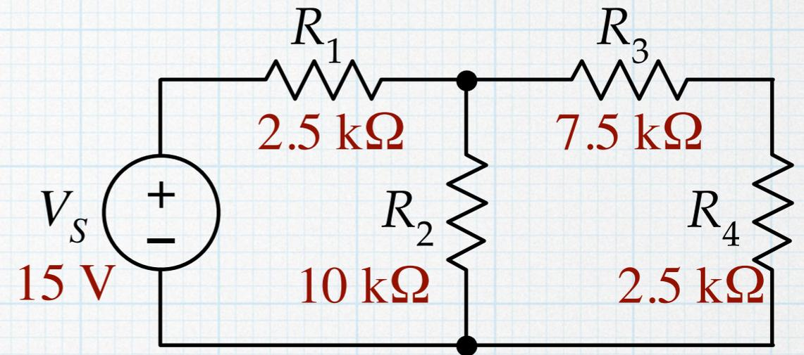
**Step 1** – Identify the nodes in the circuit. Four in this case.
