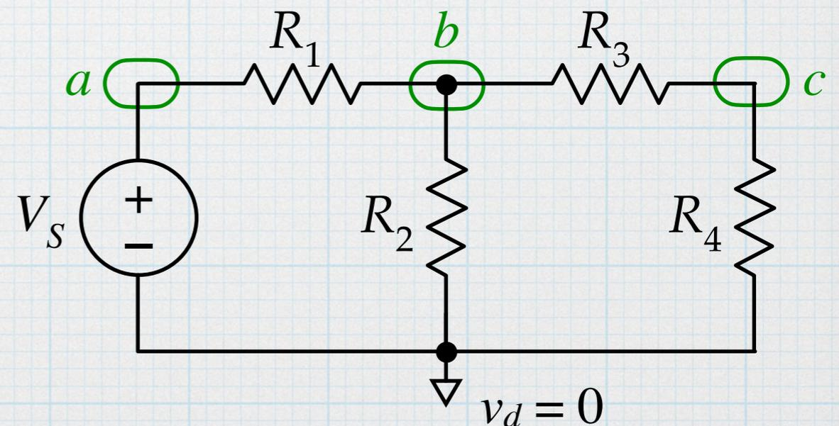
**Step 3** – Identify other nodes for which the voltage is known. As in the previous example, the voltage source causes node  $a$  to have voltage  $v_a = V_S$ .
