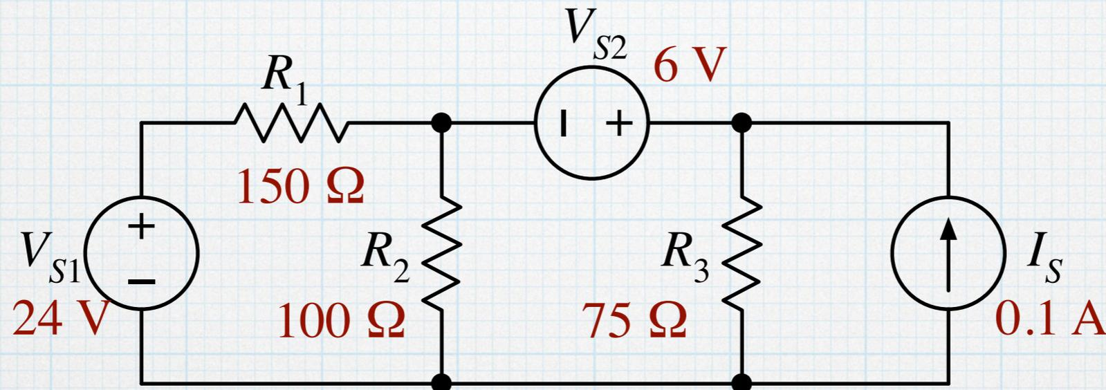
There are four nodes, and at first glance it looks like another routine application of the method. The complication arises in choosing which node to be ground. There are two voltage sources, and they do not share a node. We need to pick a ground, and we will stick with past habit and put it at the bottom node.
