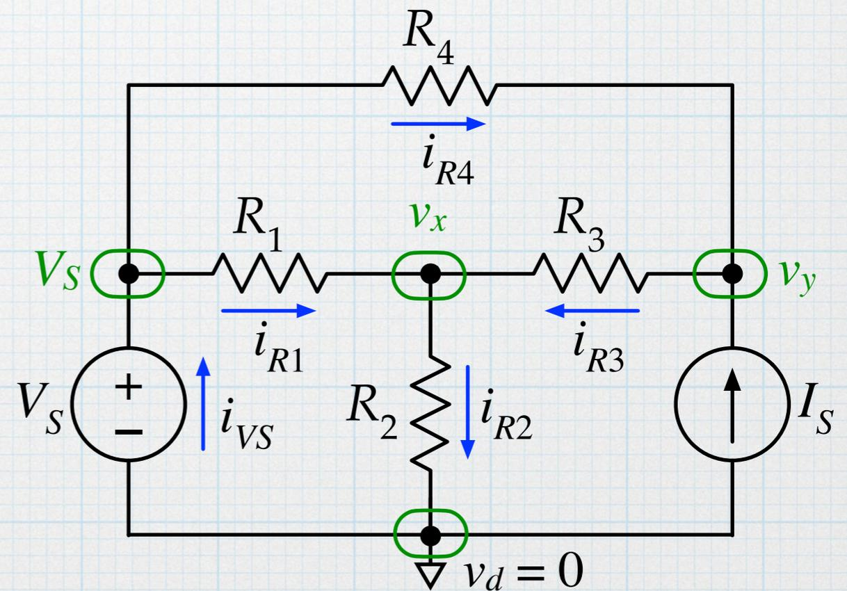
The currents that enter and leave the two unknown nodes are  $i_{R1}$ ,  $i_{R2}$ ,  $i_{R3}$ ,  $i_{R4}$ , and  $I_S$ . Note that the troublesome  $i_{VS}$  won't be involved, since it does flow into or out of of an unknown node. This is good!
