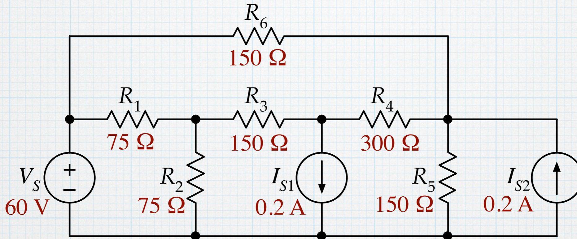
We see that there are five nodes. Choose the ground connection — the nodes on either side of the voltage source are good options. Choosing the bottom node as ground makes the voltage at the left-hand node equal to  $V_S$ .
