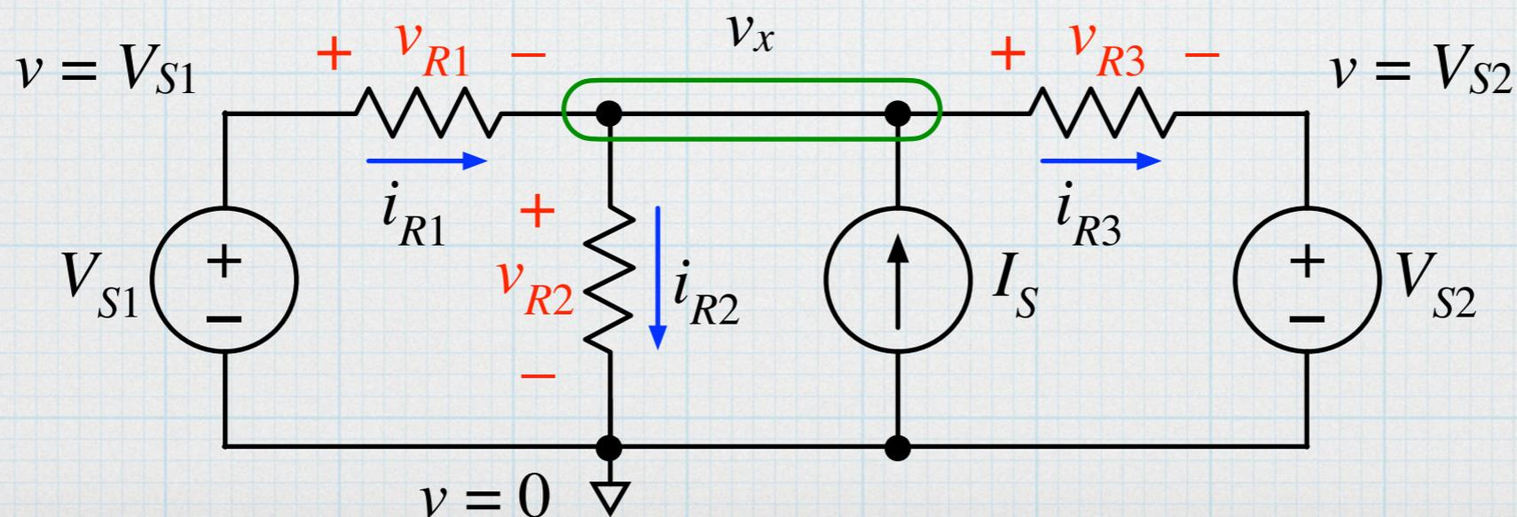
There are no series/parallel simplifications, so we can jump directly to writing the KCL equation.
