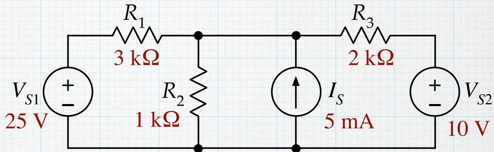
We see that there are four nodes in the circuit. Making things easier, there are two voltage sources that share a common connection. It makes sense to choose that node as ground. The ground and the two voltage sources mean that we already know the voltages of three of the nodes. This becomes a “one-node” circuit and should be easy to solve.
