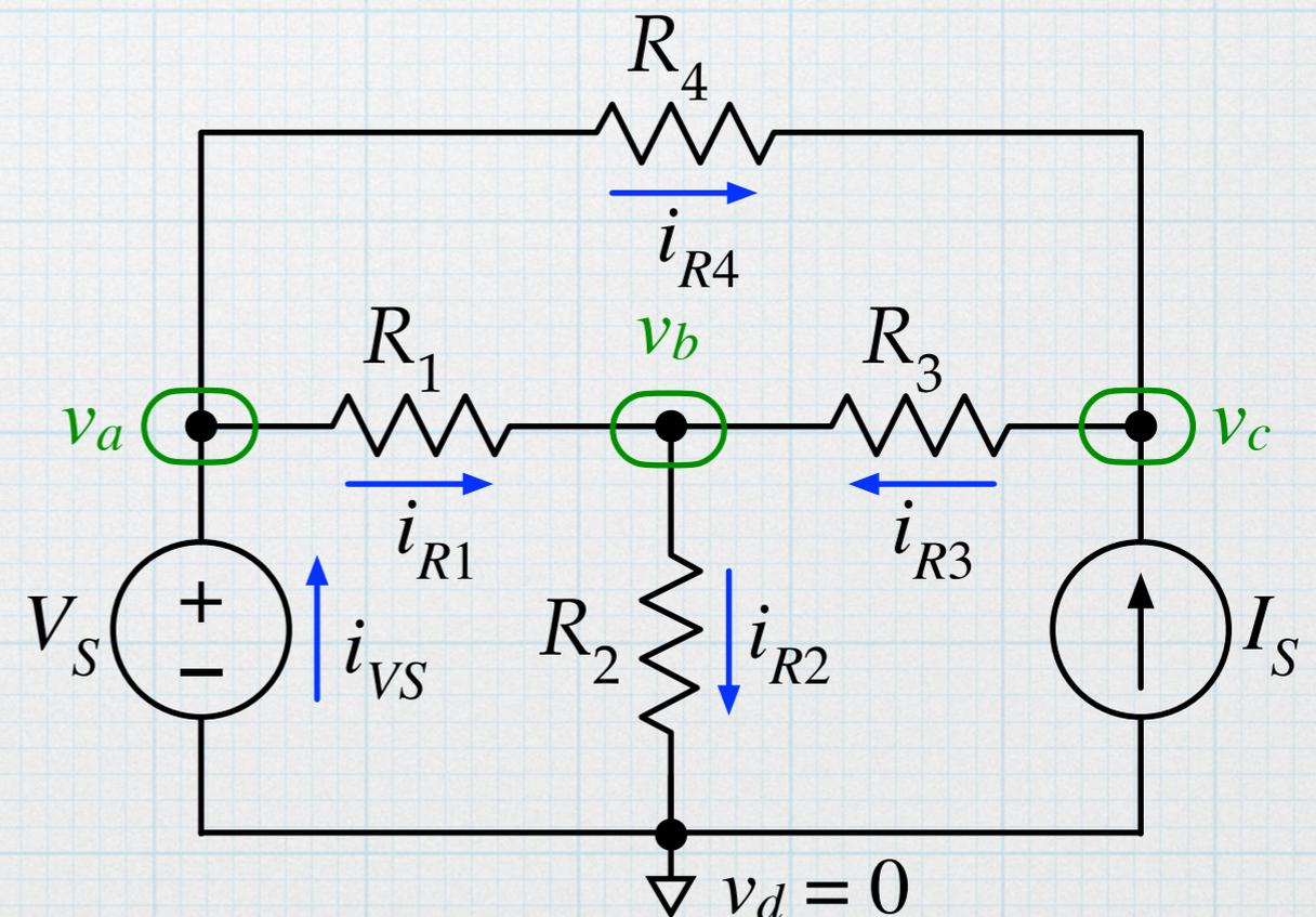
Choosing a ground node to serve as a voltage reference has two significant effects on the set of equations that describe the circuit. The first is that, since the voltage at  $d$  was assigned to be zero, it is no longer “unknown” and our math problem reduces to a set of four equations with four unknowns —  $v_a$ ,  $v_b$ ,  $v_c$ , and  $i_{VS}$ . The set can be solved!
