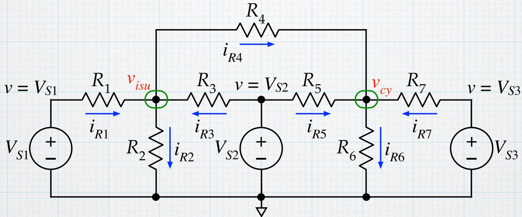
Write the KCL equations at the two nodes:
