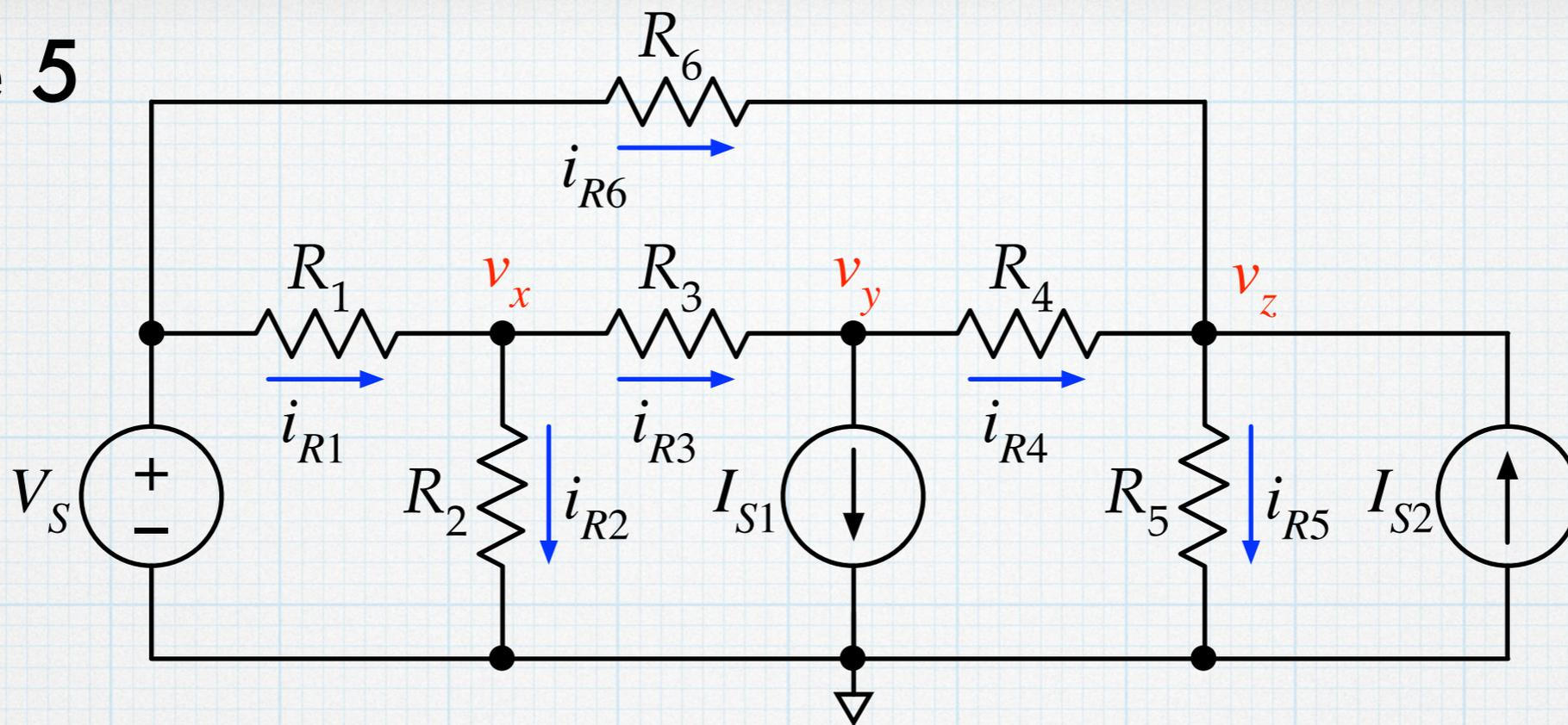
That leaves three unknown node voltages. Those are labeled as above, along with currents in each of the branches connected by nodes. Write KCL equations for the currents at each of the nodes and then convert them to node-voltage equations.
