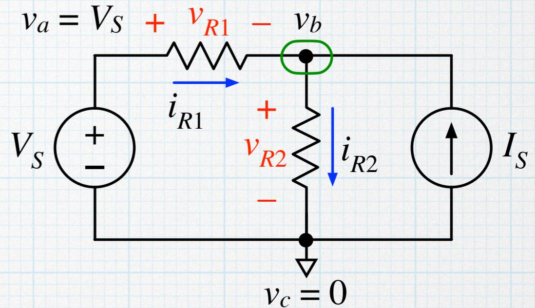
**Step 7** – Write KCL equations relating the currents at each of the unknown nodes. In this case, there is only one equation.
