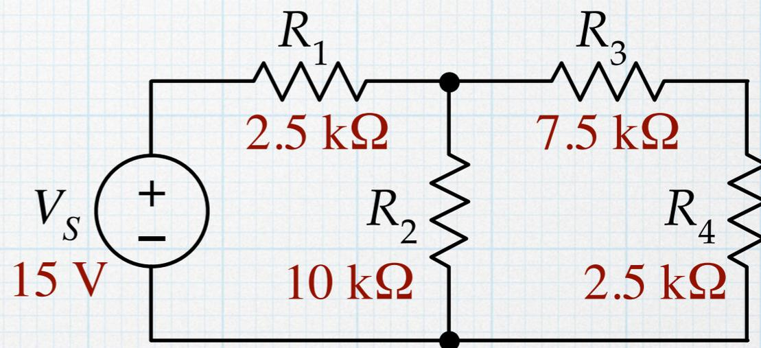
$$V_S - v_b = \frac{R_1}{R_2} v_b + \frac{R_1}{R_3} (v_b - v_c)$$
