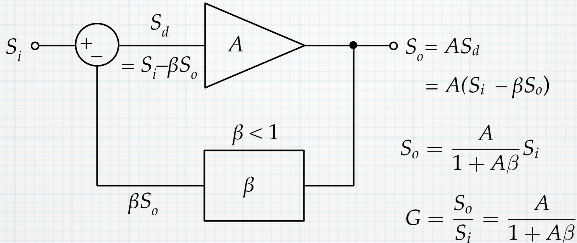
Start with an amp – large gain, but not very precise ( $A$  = “open-loop” gain)
