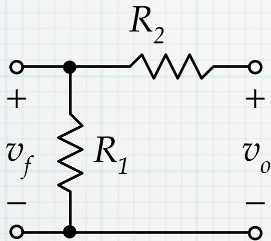
$$v_f = \frac{R_1}{R_1 + R_2} v_o$$
