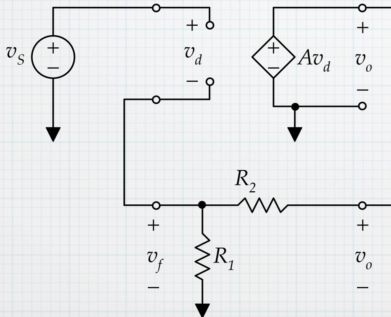
$v_d$  is the difference voltage:  $v_d = v_s - v_f$ .
