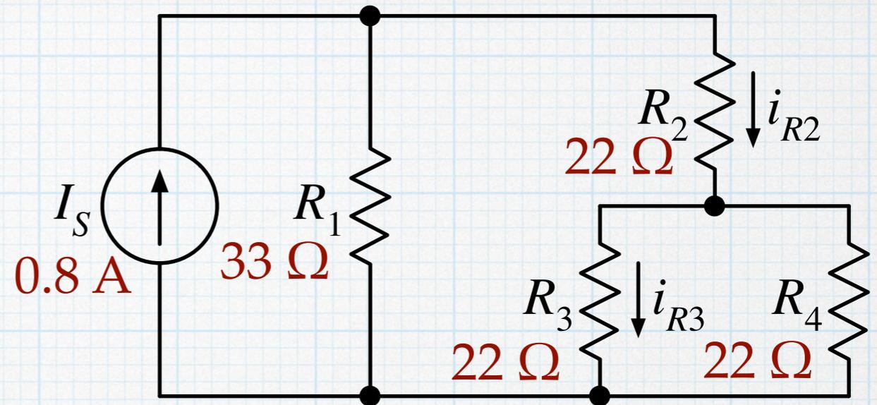
$I_S$  splits between  $R_1$  and the branch with  $R_2$ ,  $R_3$ , and  $R_4$ . To find the current through  $R_2$ , we use the equivalent resistance of that branch, which forms a current divider with  $R_1$ . Then  $i_{R2}$  is divided between  $R_3$  and  $R_4$ .
