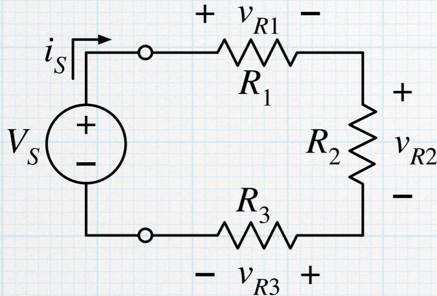
$$v_{R2} = \frac{R_2}{R_1 + R_2 + R_3} \cdot V_S$$
