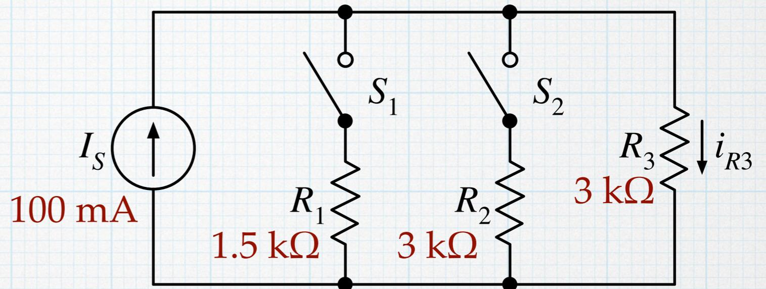
$S_1$  open and  $S_2$  open:  $i_{R3} = I_S = 100 \text{ mA}$
