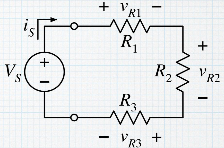
We could start by finding the current, which would be equal to the source voltage divided by the equivalent resistance of the string.
