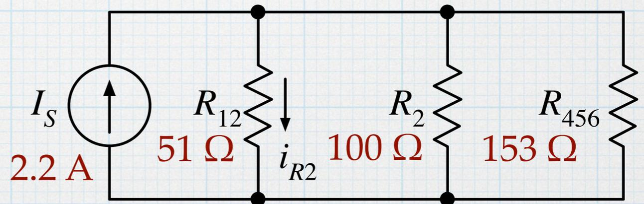
$$i_{R2} = \frac{\frac{1}{R_{12}}}{\frac{1}{R_{12}} + \frac{1}{R_3} + \frac{1}{R_{456}}} \cdot I_S = 1.19 \text{ A}$$
