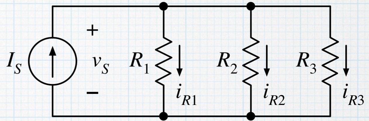
We could start by finding the voltage, which would be equal to the source current multiplied by the equivalent resistance of the parallel resistors.
