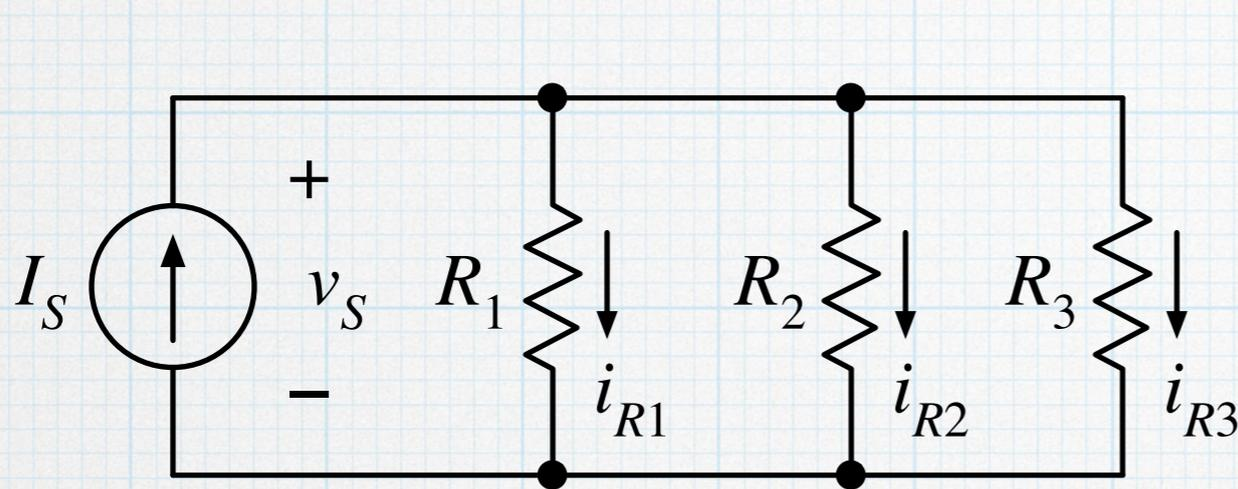
$$i_{R1} = \frac{\frac{1}{R_1}}{\frac{1}{R_1} + \frac{1}{R_2} + \frac{1}{R_3}} \cdot I_S$$
