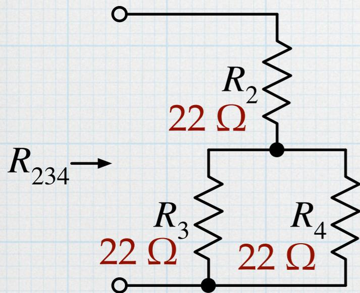
$$R_{234} = R_2 + R_3 \parallel R_4$$
