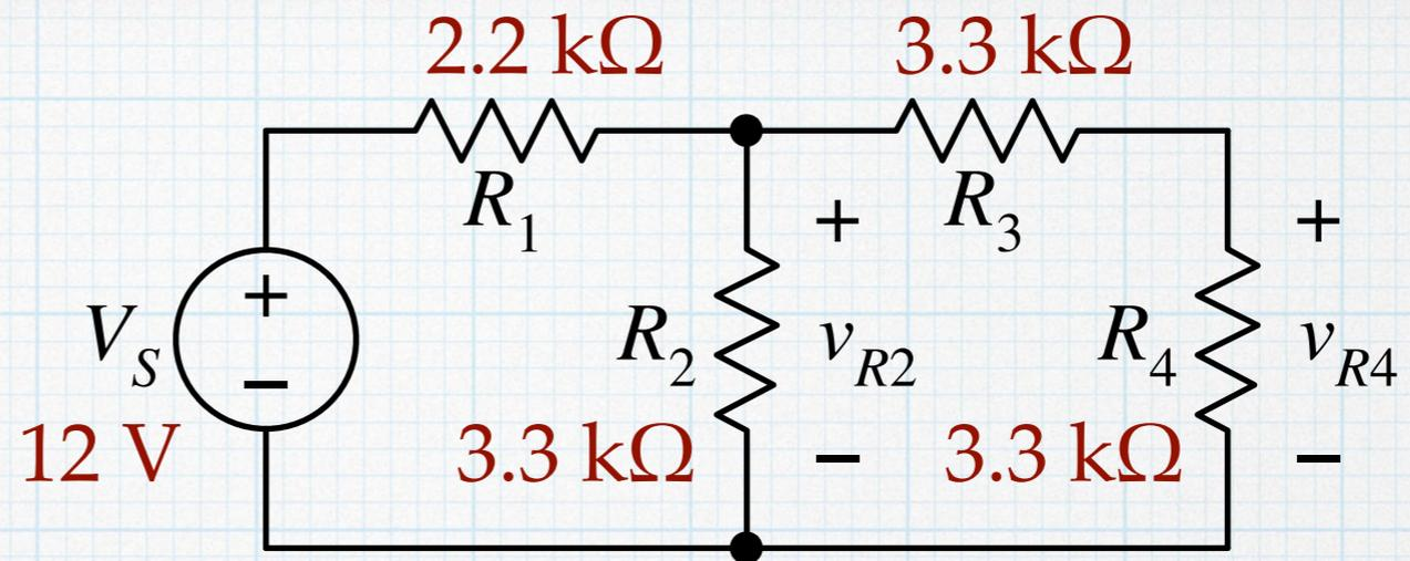
We solve this using the voltage divider calculation twice in succession. First we find  $v_{R2}$  using a voltage divider formed by  $R_1$  and the equivalent resistance of  $R_2$  in parallel with the series combination of  $R_3$  and  $R_4$ .
