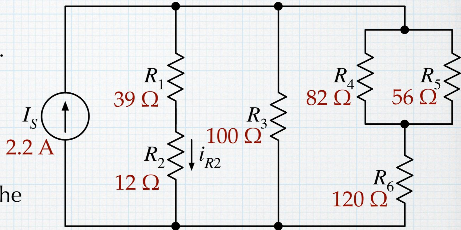
$$R_{12} = R_1 + R_2 = 51 \Omega$$
