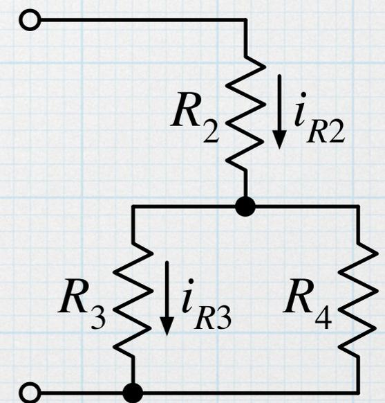
$$i_{R3} = \frac{\frac{1}{R_3}}{\frac{1}{R_3} + \frac{1}{R_4}} \cdot i_{R2} = 0.2 \text{ A}$$
