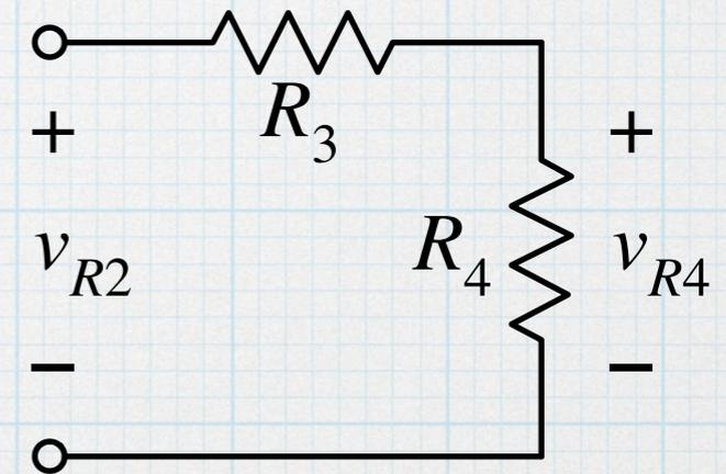
$$\begin{aligned} R_{234} &= R_2 \parallel (R_3 + R_4) \\ &= (3.3 \text{ k}\Omega) \parallel (6.6 \text{ k}\Omega) \\ &= 2.2 \text{ k}\Omega \end{aligned}$$
