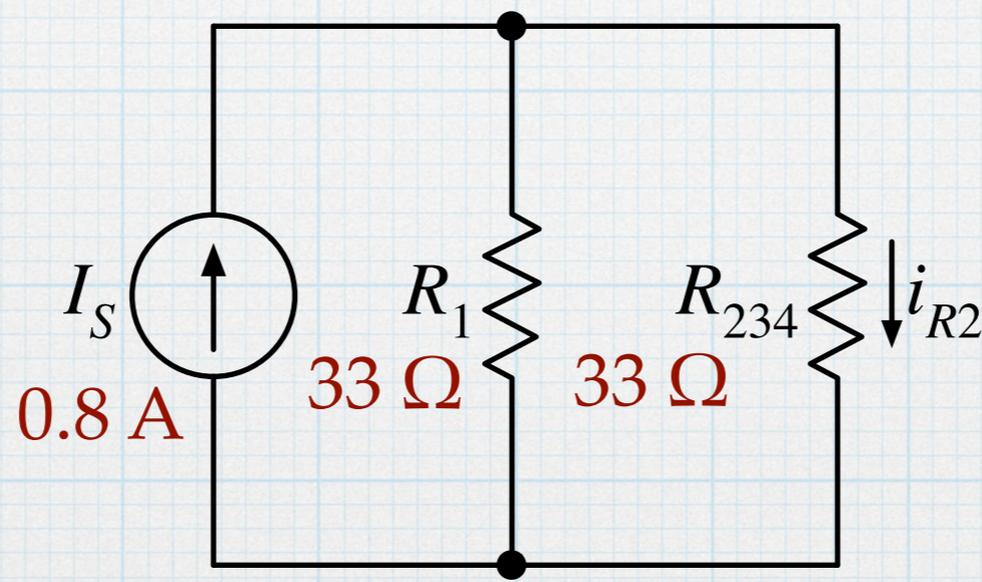
$$i_{R2} = \frac{\frac{1}{R_{234}}}{\frac{1}{R_1} + \frac{1}{R_{234}}} \cdot I_S = 0.4 \text{ A}$$
