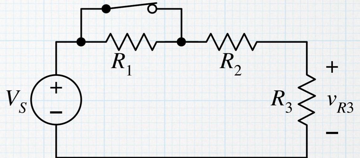
There are several approaches to answering this question, but using voltage dividers is a convenient method. With the switch closed,  $R_1$  is shorted out and
