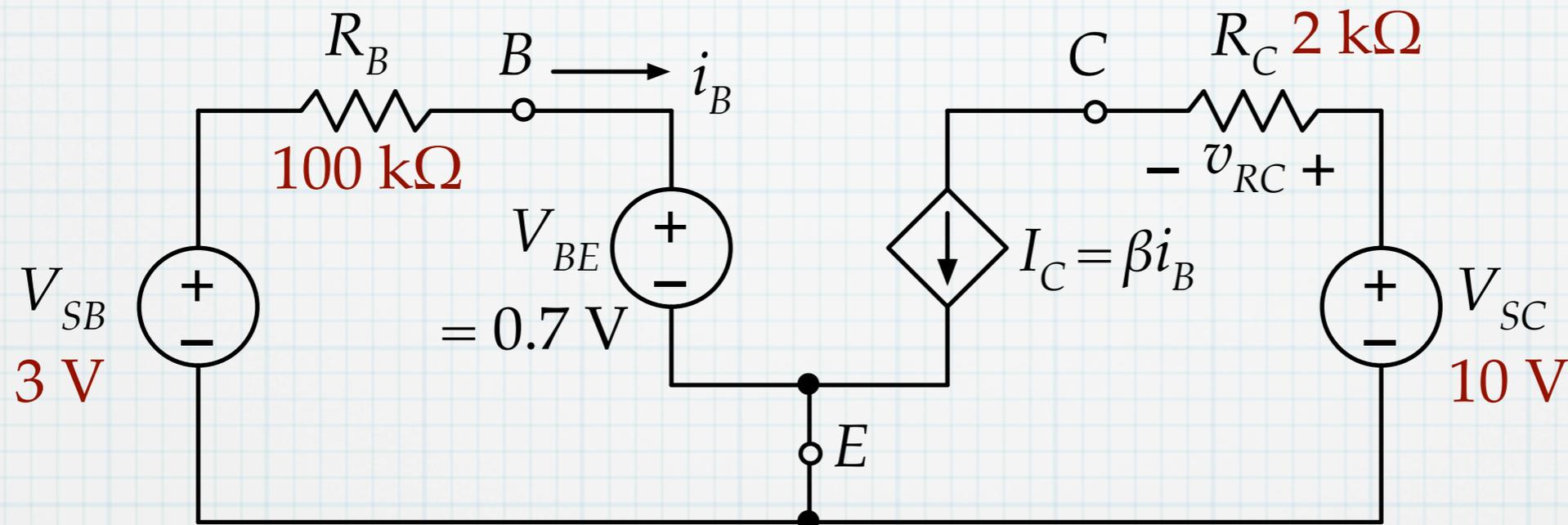
Around the left-hand loop:  $V_{SB} - i_B R_B - V_{BE} = 0$ .
