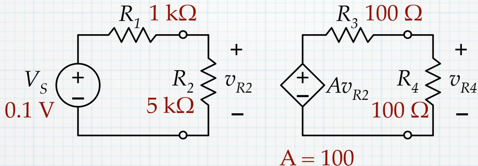
Find an expression for  $v_{R4}$  using a voltage divider
