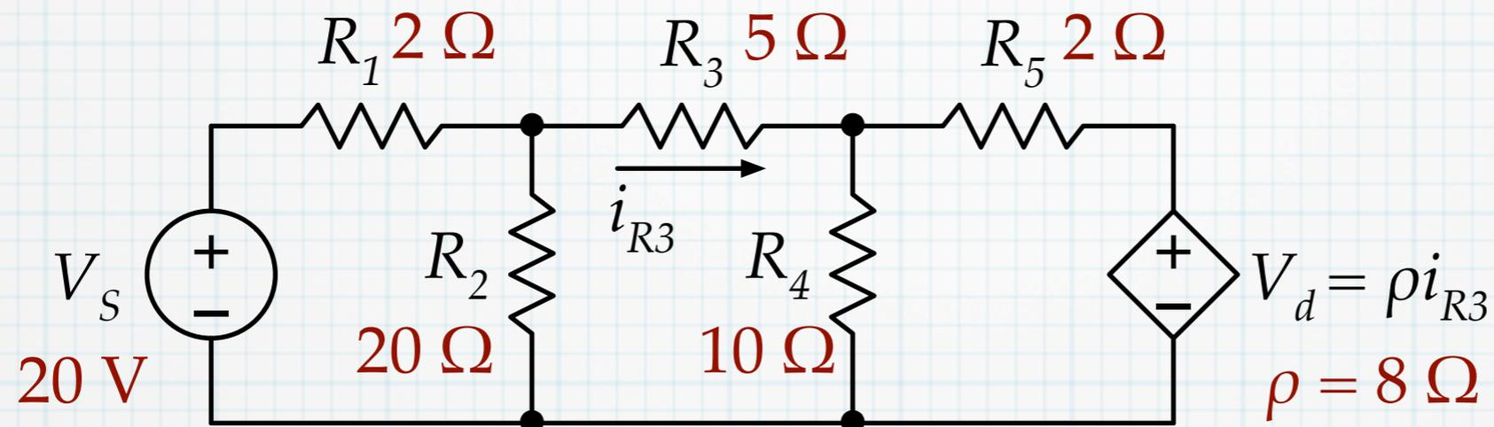
Use the node-voltage method. Define ground at the bottom and identify the unknown nodes. Initially, treat  $V_d$  as if it were known. We will write node equations for  $v_a$  and  $v_b$ , and then we add an *auxiliary* equation to handle  $V_d$ .
