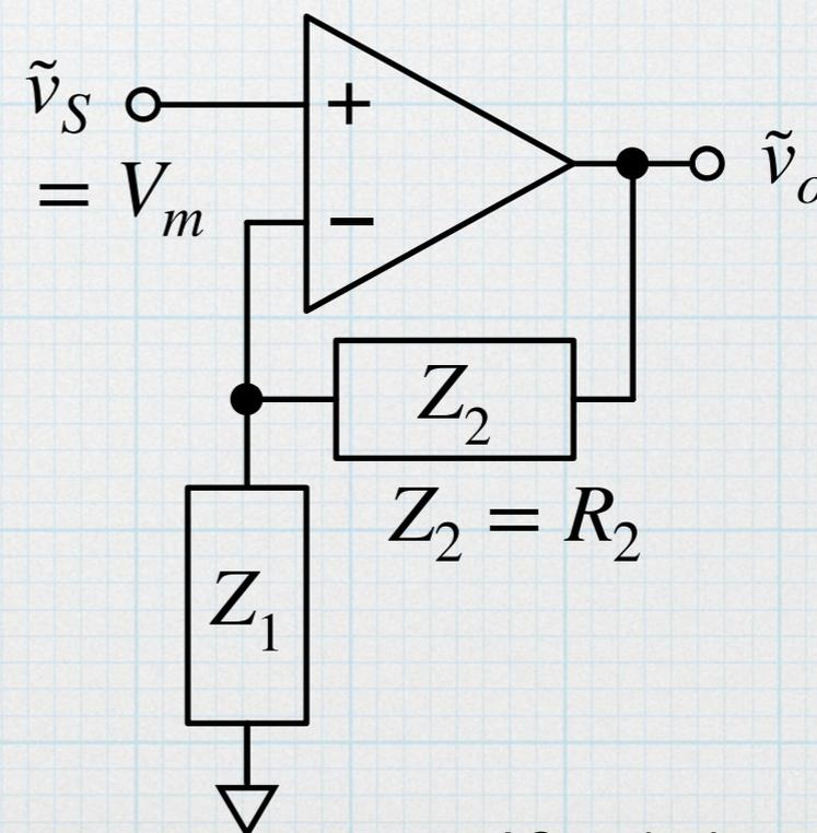
$$G = 1 + \frac{Z_2}{Z_1} = 1 + \frac{R_2}{R_1 + \frac{1}{j\omega C}} \quad \text{Proceed with caution.}$$
