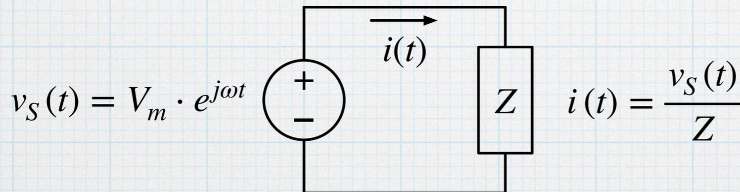
$$\text{resistor: } Z = R \quad \text{capacitor: } Z = \frac{1}{j\omega C} \quad \text{inductor: } Z = j\omega L$$
