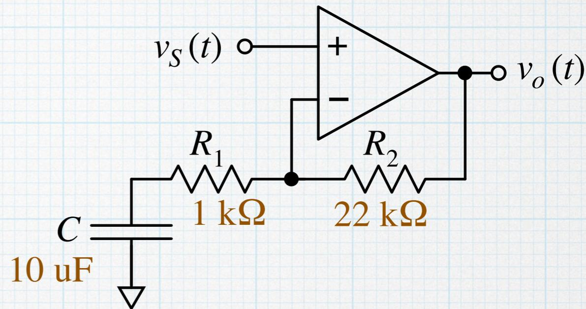
It may not be immediately obvious that this is a non-inverting amp, but if we treat the  $R_1$ - $C$  series combination as a single impedance, we can draw the complex version of the circuit. Then it is familiar.
