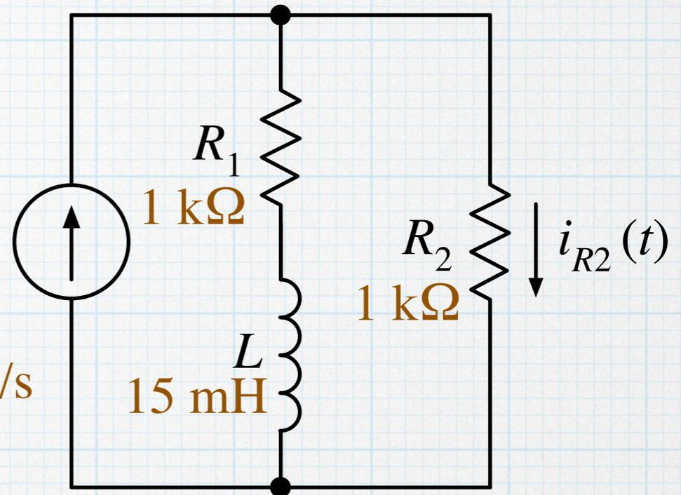
Again, we have a simple current divider if we treat the  $R_1$ - $L$  series combination as a single impedance.
