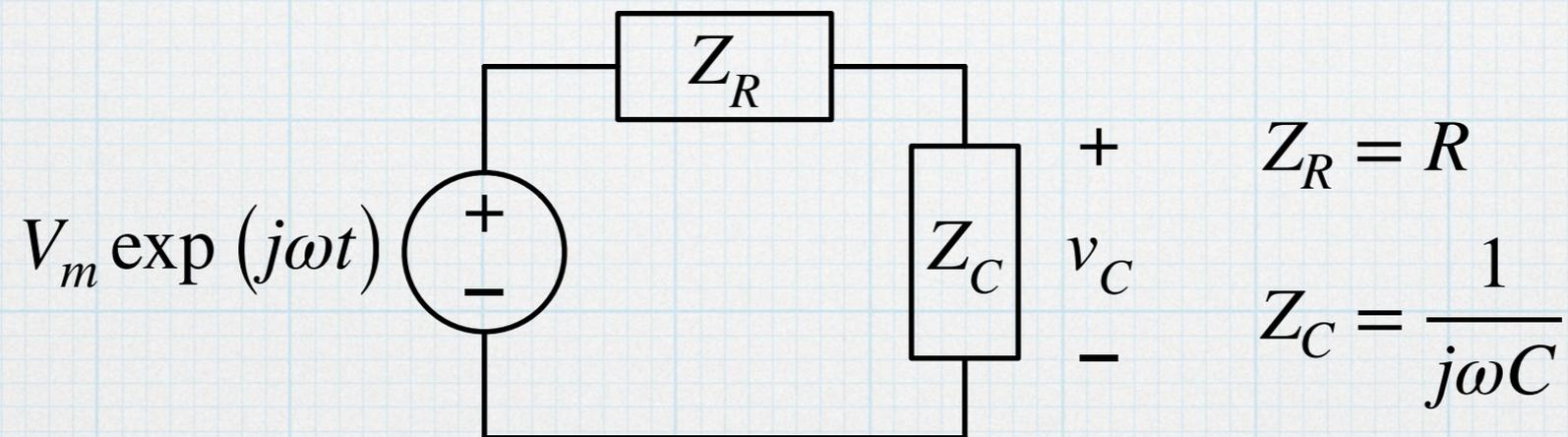
In viewing the complex circuit and thinking about how to approach it if the impedances were all resistors, it seems that using a voltage divider would be a reasonable approach.
