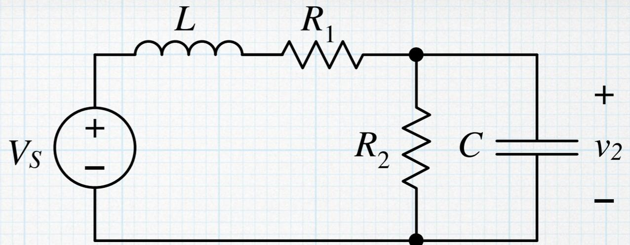
Suppose the frequency is very low,  $\omega \rightarrow 0$ . (i.e. DC.) The inductor behaves like a short and the capacitor like an open.
