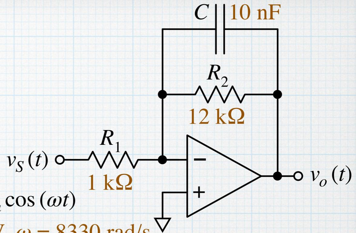
How do ops amp work in a complex circuit? Just like they did before. The rules are unchanged: no current flows into the input,  $\tilde{i}_+ = \tilde{i}_- = 0$ , and when there is a negative feedback loop,  $\tilde{v}_+ = \tilde{v}_-$ .
