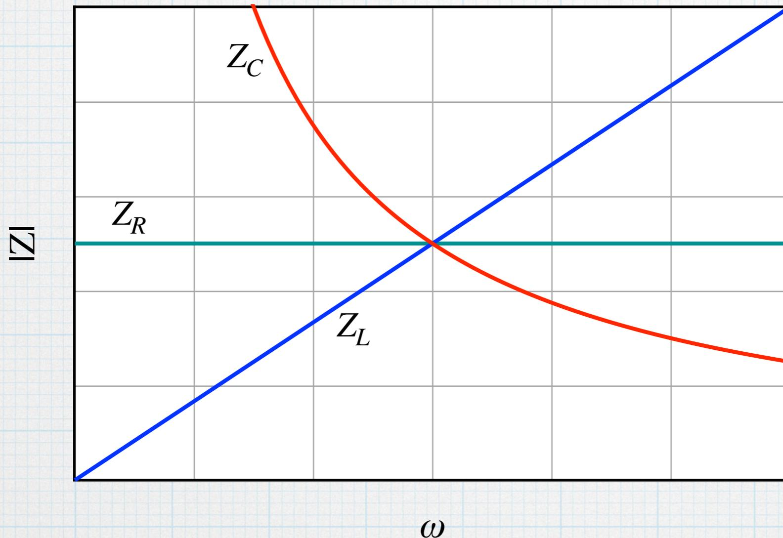
Resistors are frequency independent. Capacitors and inductors change behavior as the frequency changes.
