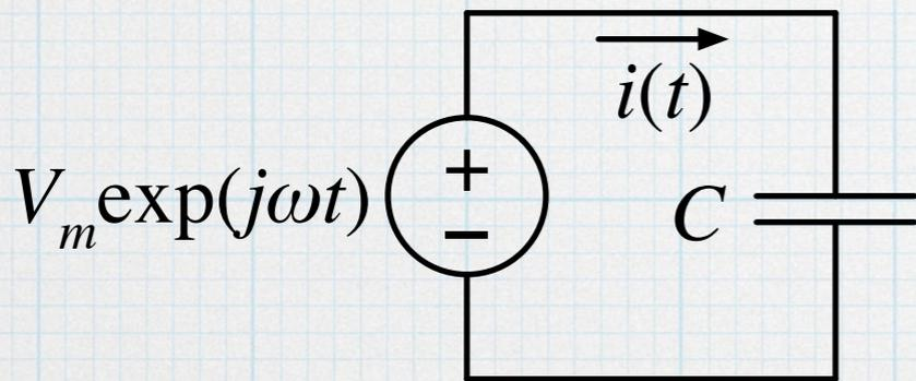
$$i_C(t) = C \frac{d(V_m e^{j\omega t})}{dt} = j\omega C [v_C(t)]$$
