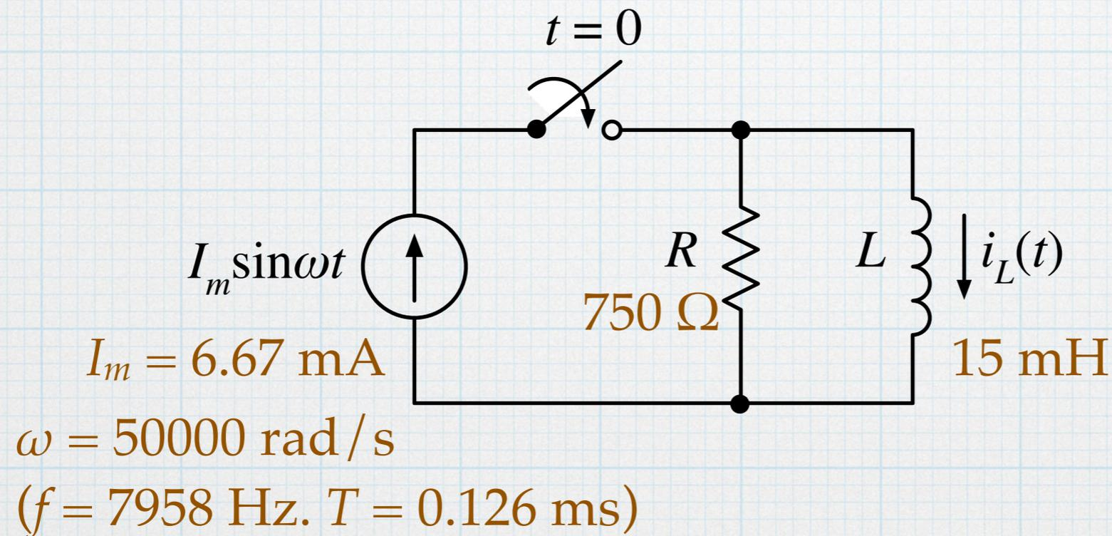
In the circuit, the switch closes at  $t = 0$ . The inductor current is zero for  $t < 0$ , and so the initial condition is  $i_L(t = 0) = 0$ .
