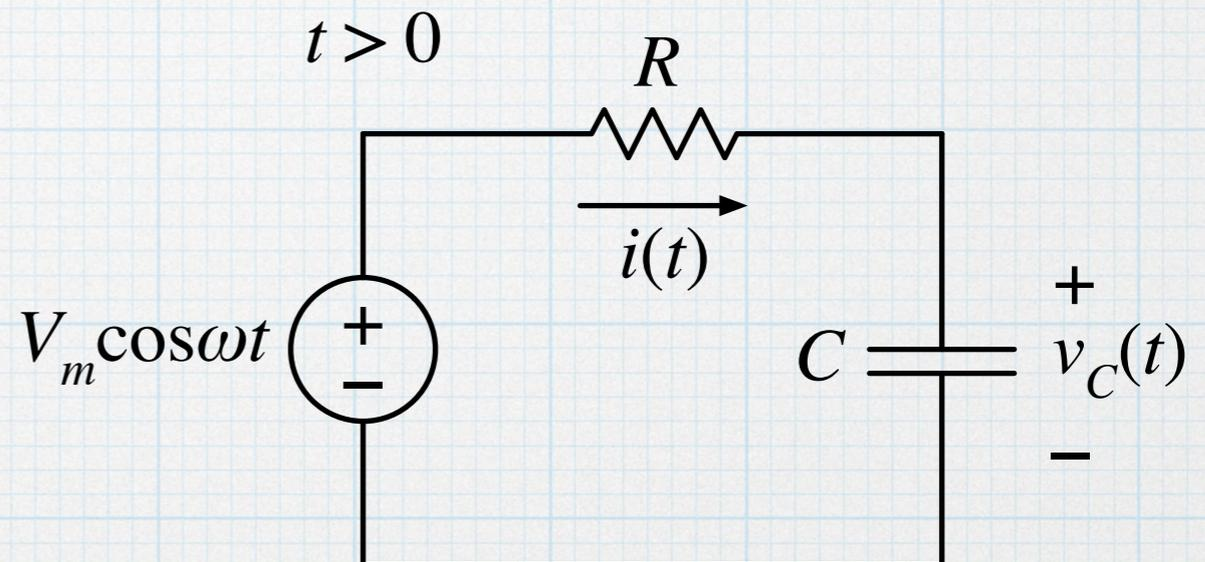
Use the two-solution approach:  $v_c(t) = v_{tr}(t) + v_{ss}(t)$ .
