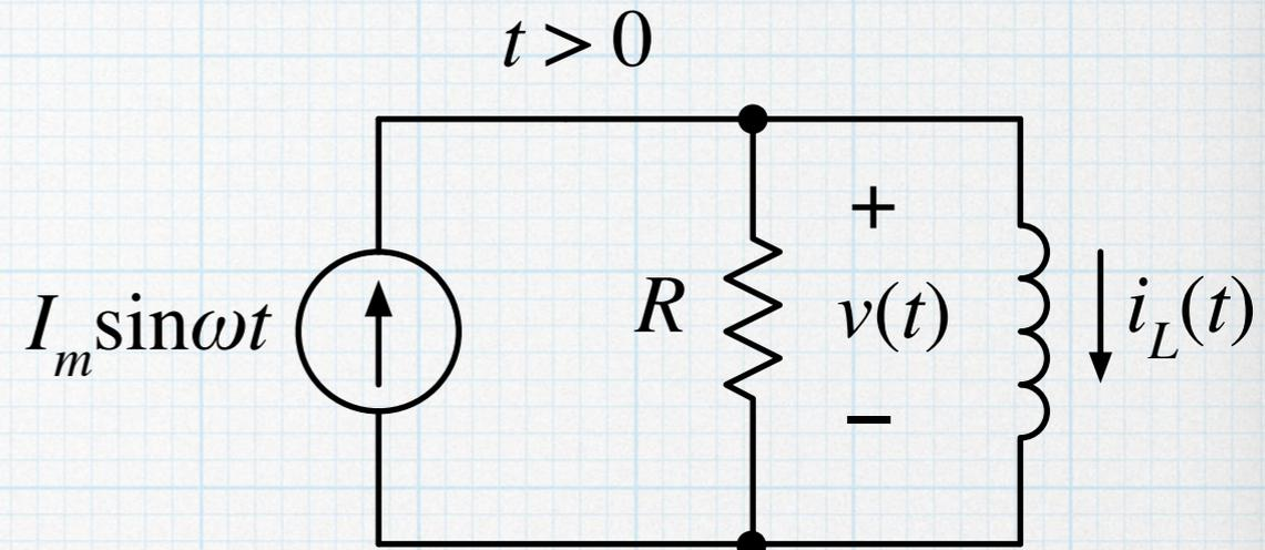
$$i_L(t) = A \cos \omega t + B \sin \omega t + D \exp\left(-\frac{t}{\tau}\right) = M \cos(\omega t - \theta) + D \exp\left(-\frac{t}{\tau}\right)$$
