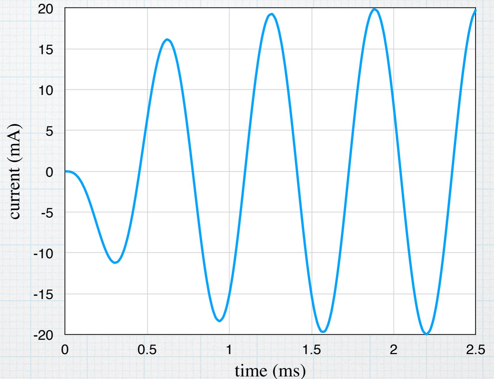
At the start the current is small, but it builds up with each cycle. With a time constant of 0.4 ms, the transient is essentially complete by 2 ms. After that, the current oscillates at the source frequency (which is the resonant frequency of the circuit), with an amplitude of 20 mA, corresponding to the resistor voltage of 10 V and inductor and capacitor voltages of 20 V.
