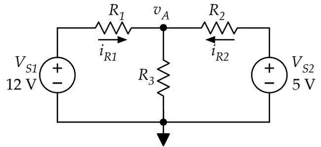
Build the circuit and perform measurements to confirm that it meets the design goals. The voltage and currents don't have to be exact, but they should be within 5% of the specifications.
