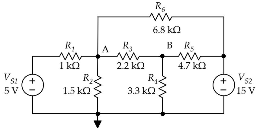
Figure 3. Node-voltage circuit C.
