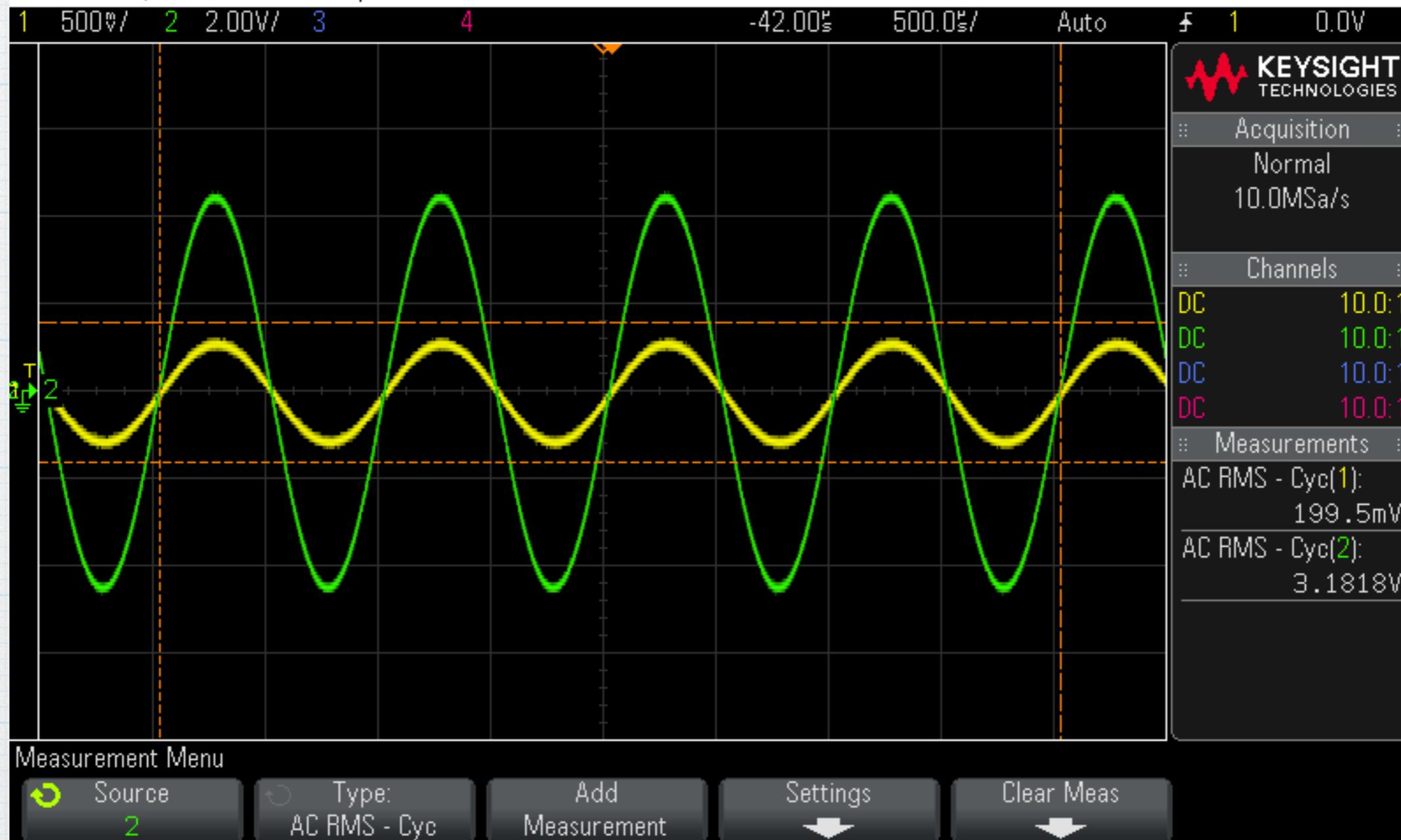
$$G = \frac{v_o}{v_i} = \frac{3.18 \text{ V}}{0.200 \text{ V}} = 15.9$$
