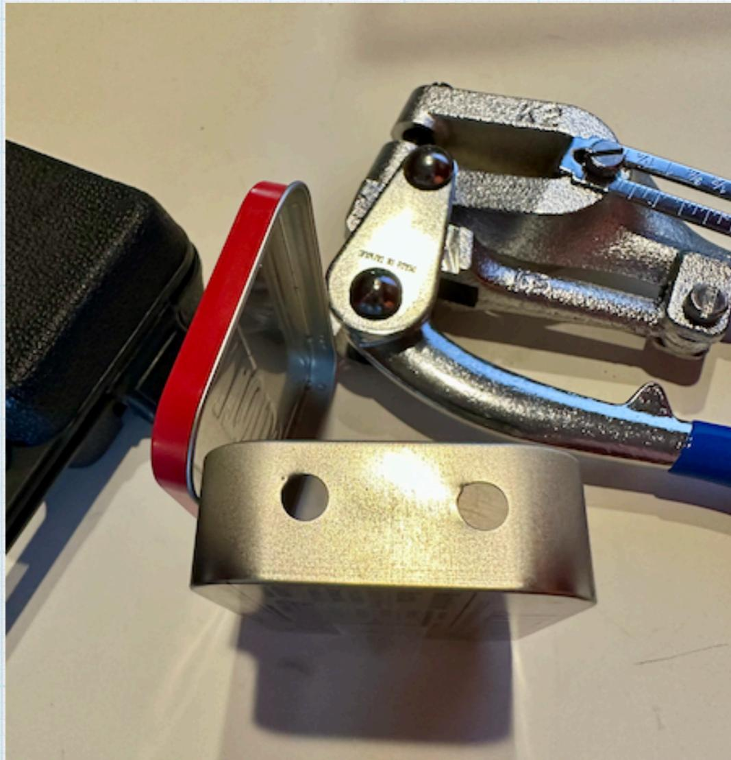
Since the holes are offset slightly from the center, it might be necessary to nip two small chunks out of the lid in order to have it close completely.
