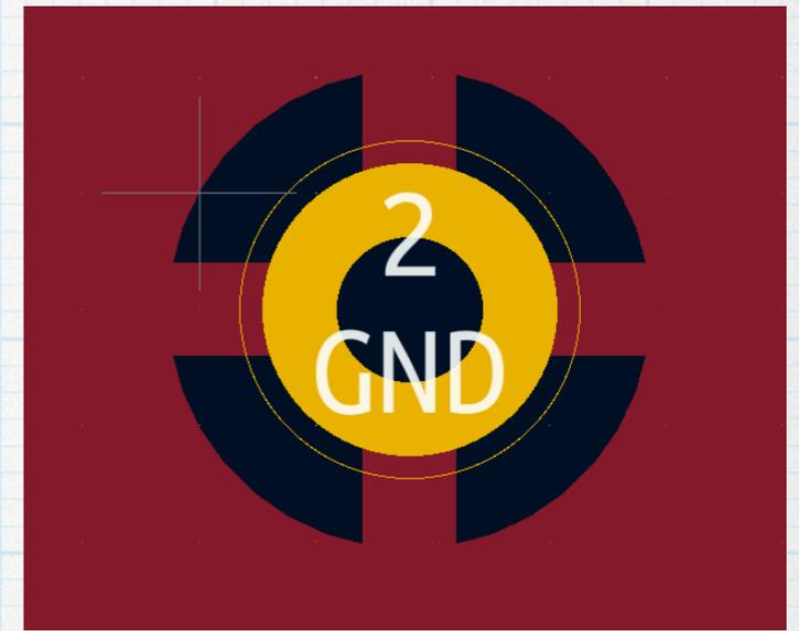
The thermals help, but it will still be more difficult to make solder connections to the ground plane. It will be necessary to get more heat into the connection to melt the solder. Things to do:
